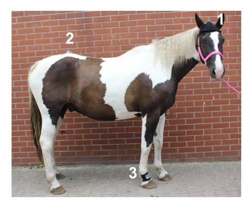
**Fig.1**: Horse instrumented with the inertial sensor system: accelerometer at the head (1), accelerometer at the pelvic (2) and gyroscope sensor for the right forelimb (3). *Pferdeheilkunde*, 30 (2014) p. 646.
