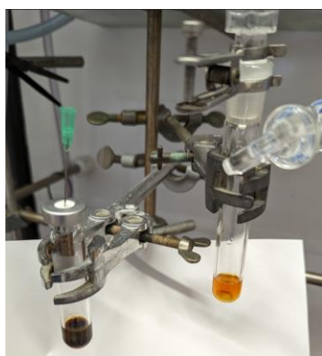
Figure 3.10: Color of the reaction mixture after 20 h at 70 °C using microwave heating (left) and conventional heating (right).
