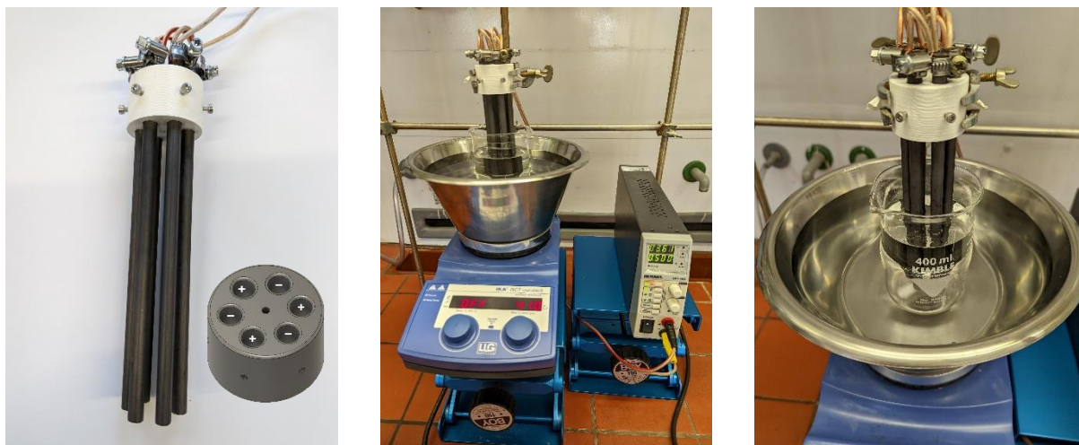
Figure 5.1: From left to right: 1) Electrode configuration using 8.2 mm graphite rods in a 3D-printed PLA-Holder (STL-File in the attachments); 2) Reaction setup with lab power supply and 400 mL glass beaker 3) Close-up of the reaction solution.
