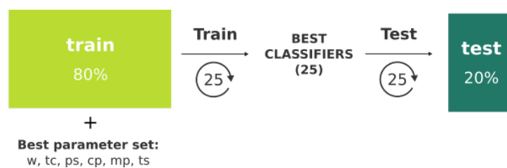
FIGURE 5.4: Training and testing scheme: (1) First the original data set is divided into training and test fractions. Next, the training and testing fractions are separately pre-processed. (2) The normalized training fraction is further used to tune parameters of the GA and the weight w in an inner 5-fold cross-validation. (3) The best parameter set is further applied to train classifiers on pre-processed training fraction and evaluated on the hold-out test data set.
