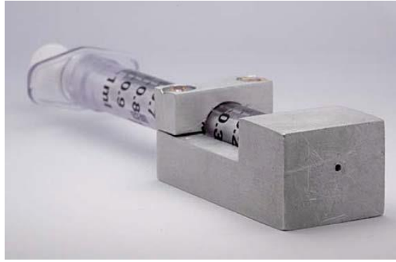
Figure 4 Syringe- die device as a lab- scale ram extrusion introduced by Ghalanbor et al. (left) [29].
