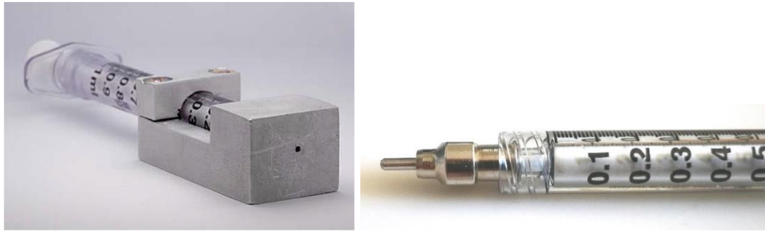
Figure 15 Syringe-die device as a lab-scale ram extrusion introduced by Ghalanbor et al. (left) [29] and adapted lab- scale extrusion device with luer lock die (right).
