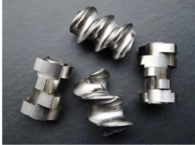
Figure 8 Kneading- and conveying elements of modular extruder screws, picture adapted from [51].
