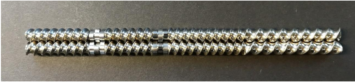
Figure 16 Modular extruder screws of the ThreeTec ZE9.
