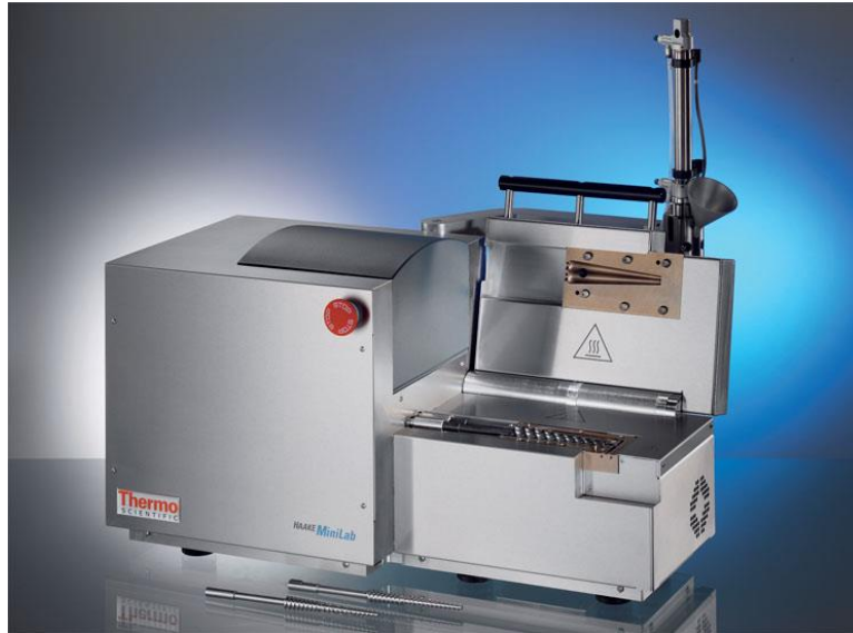
Figure 7 Example of a twin-screw extruder, Haake MiniLab Compounder (Thermo Scientific, Karlsruhe, Germany), adapted from [50].
