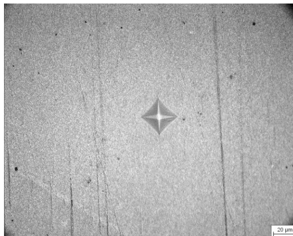
Fig. 29: Indent on TZ-3Y single layer
