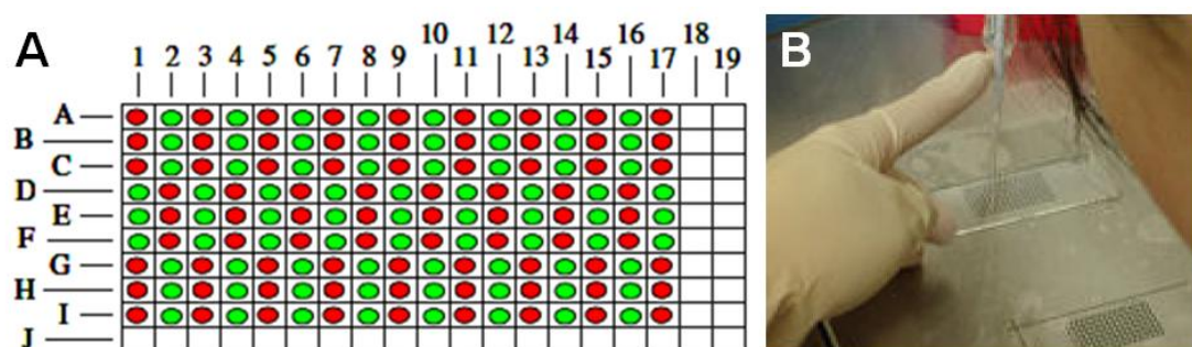
Figure 10. Manual spotting. (A) An example of the grid lattice used for manual spotting with the pattern of 1.5 \times 1.5 mm square. Therefore the distance between spots was set to 1.5 mm. (B) The procedure of manual spotting. Slides were put on top of the grid lattice, and long tips were used for spotting.
