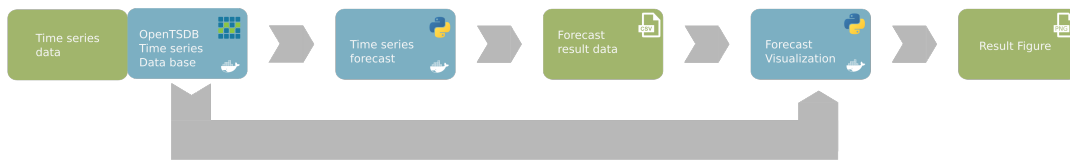
Figure 4.9: The figure shows the integration of a time series database with a convolutional Long-Short-Term Memory network for time series forecasts. The blue boxes represent the different parts of the process, including the forecast visualisation, which is achieved by querying the original data from the database and plotting it together with the forecast. This separation allows for a more comprehensive analysis and a better understanding of the data. The resulting graph can be seen in Figure 4.10.
