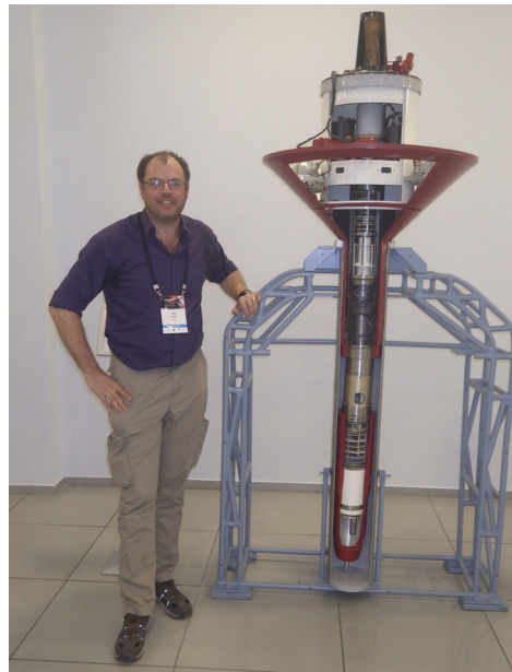
Fig. 5 Model of one of the Lunar-A penetrators, never flown. Only the black element at left would penetrate into the regolith to perform seismic and heatflow studies: the formidable propulsion and attitude control hardware necessary to orient and decelerate the vehicle to survivable impact speed is evident at right, Photo: R. Lorenz
