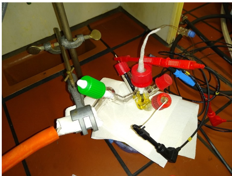
Fig. S54: General set-up for bulk electrolysis experiments.
