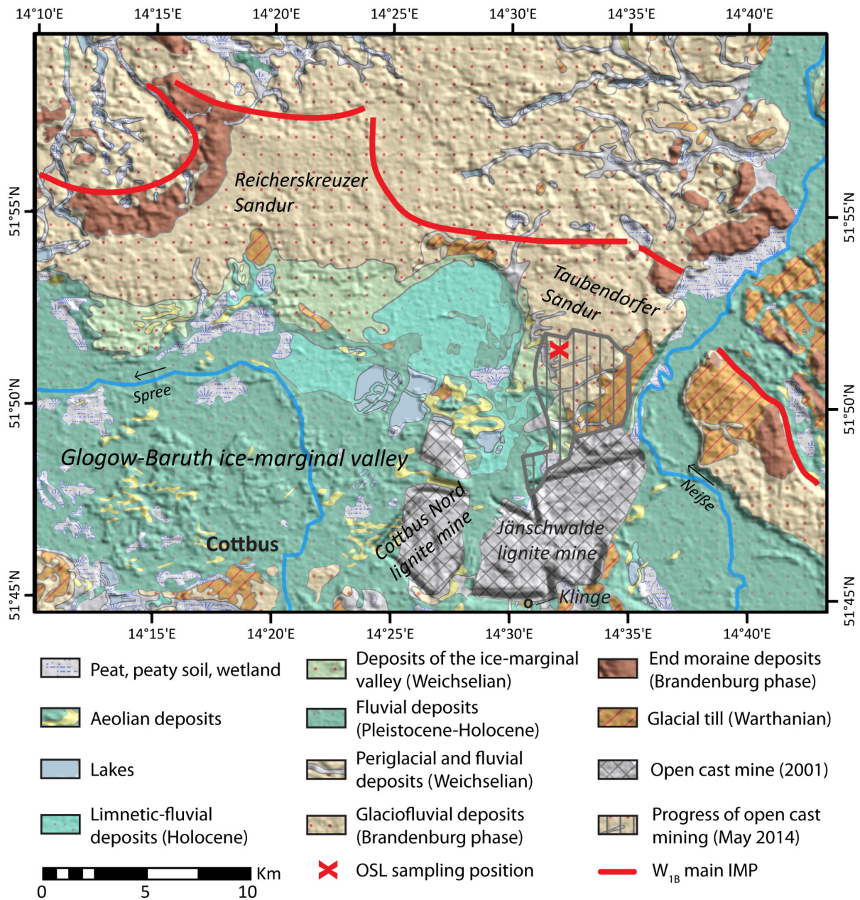
Fig. 44: Geological overview map of the study area. Geological data simplified after Lippstreu et al. (2001). W 1B main IMP compiled after Marcinek (1961) and Liedtke (1981). Hillshade based on SRTM data (Jarvis et al., 2008).
