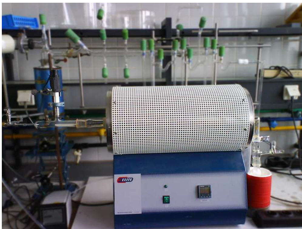
Figure 2.1. The pyrolysis apparatus used to prepare corannulene 1 . Left: Nitrogen-inlet, pressure gauge and sample boat. Right: Cold trap immersed in liquid nitrogen and connection to vacuum pump.
