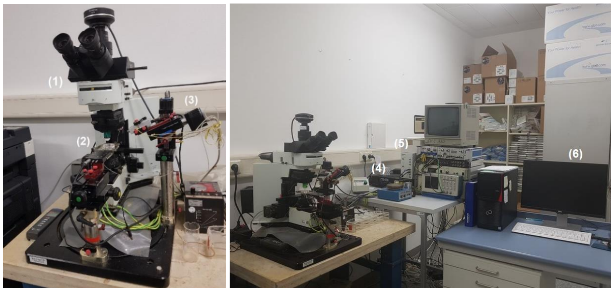
Figure 9: Setup of the fluorescence calcium imaging. Located at the Charité University of Medicine – Campus Virchow Clinic, Department of Ophthalmology, Berlin, Germany. (1) Digital Olympus XM-10 camera, (2) coverslips on inverted microscope stage, (3) micromanipulator, (4) LED-Hub light source, (5) Omicron controller, (6) computer with digital imaging software system. [Images by E. Turan].
