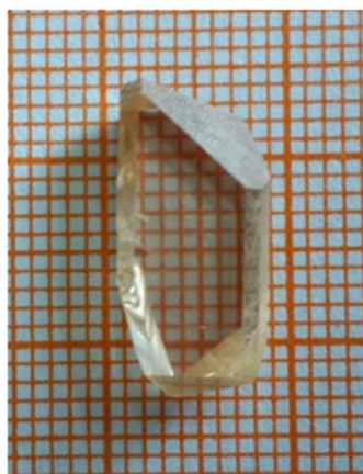
Fig. 2.13 As-grown MgW crystal with 0.89 at. % Tm-doping.
