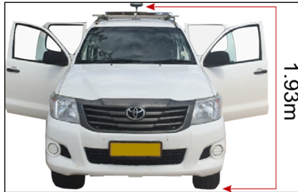
Figure 2-6: Measurement setup – Toyota Hilux with GS 16 sensor on the car roof (photo & editing: Robert Arendt 2018).
