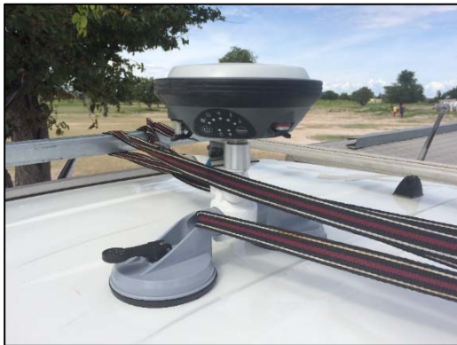
Figure 2-5: Leica GS 16 Sensor installed on the roof of a car (photo: Robert Arendt 2018).
