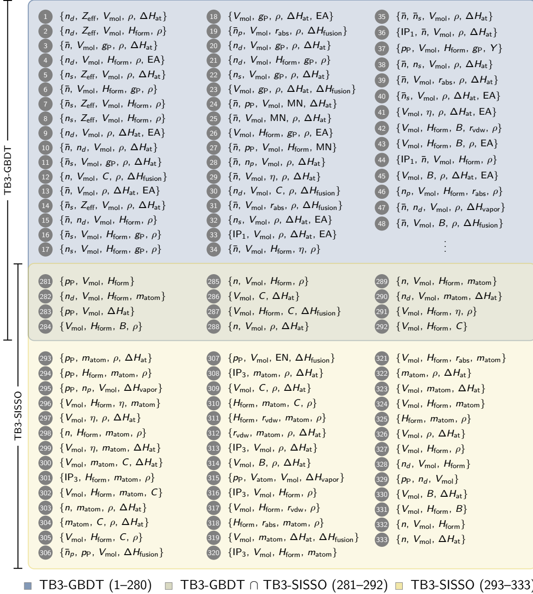
Fig. 5.19. Identified minimally non-redundant (sub-optimal) feature subsets for the prediction of the bulk modulus K_{\text{VRH}} in the Voigt-Reuss-Hill notation [485] using the tolerance-based branch-and-bound algorithm (TB3) and GBDT or SISSO as the feature-selection criterion (Section 4.1). Shown is the intersection and the union of the two feature-identification methods corresponding to a Jaccard similarity coefficient (Eq. 5.1) of 0.04. It should be noted that due to the different machine-learning algorithms, a direct comparison between TB3-GBDT and TB3-SISSO may not be appropriate. The numbering is used for referencing purposes.
