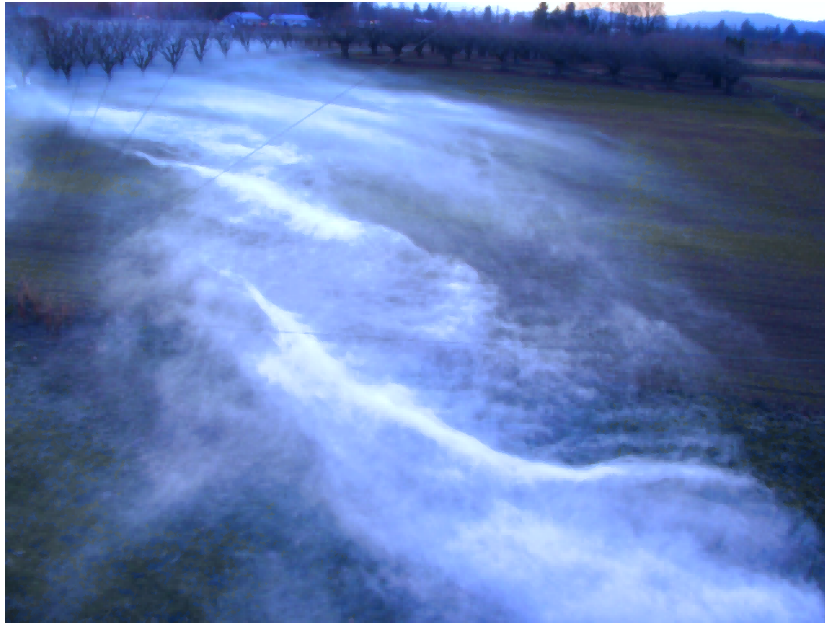
Figure 1.3: Observation of a sub-mesoscale flow structure at the surface through the fog. The fog injection occurred before sunrise, when stratification was at its highest. Such flow structures are considered non-turbulent, and their induced turbulence hypothetically leads to intermittent mixing in the boundary layer. Such mixing events are not considered by conventional models and are investigated in this work. Modified picture from http://submeso.org , used with permission of Dr. Larry Mahrt.
