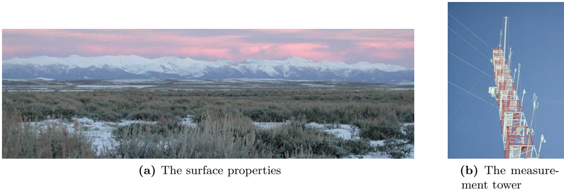
Figure 3.1: (a) The site of the FLOSS2 experiment. (b) The 30 m high measurement tower with seven mounted sonic anemometers. ©2021 UCAR.
