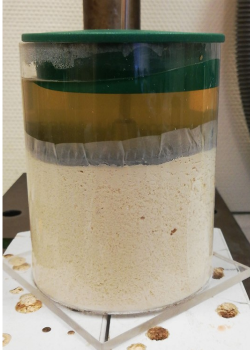
Figure 3.3: Larger phantom for IR-MRE. The press and the filter are still inside the vessel while the sample is cooling at room temperature.
