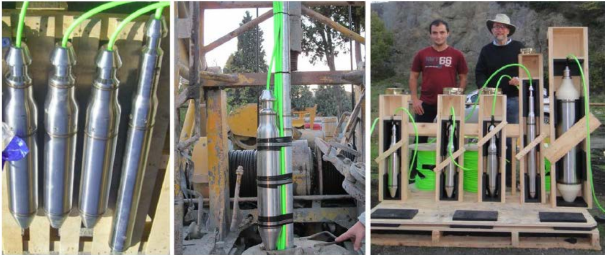
Figure 2.4: Left) Sensors of the first GONAF instrumentation at the Tuzla borehole. Right) The optimized array after the Tuzla test: from left to right are three 1 Hz vertical L4s, a sonde containing the 2 and 15 Hz 3-C, and a 1Hz 3-C L4 instrument. Center) One of the 1 Hz vertical L4 sensors banded to the cementing/installation pipe on its way downhole at the Tuzla site. (From Prevedel et al. , 2015)
