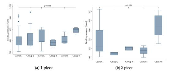
**Figure 10.** Boxplots showing the bending moment at the time point of fracture depending on dynamic loading conditions respecting the applied load and amount of cycles (as categorized in Section 2.7) for 1-(a) and 2-piece (b) zirconia implants. Whiskers are used to represent all samples lying within 1.5 times the interquartile range. Dots represent outliers. Detailed data can be found in Tables 3 and 4. No 2-piece implants were allocated to group 5.
