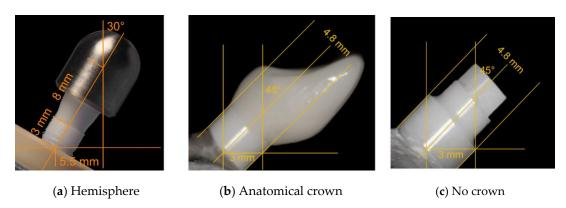
**Figure 11.** Exemplary schemes of embedded implants according to ISO 14801 (a) [21], equipped with an anatomically shaped incisor crown (b) or without any restorative supply (c) [20]. When embedding
