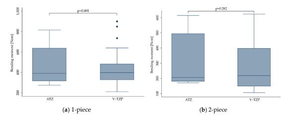
**Figure 3.** Boxplots showing the bending moment at the time point of fracture depending on the material selection for 1- (a) and 2-piece (b) zirconia implants. Whiskers are used to represent all samples lying within 1.5 times the interquartile range. Dots represent outliers. Detailed data can be found in Tables 3 and 4.
