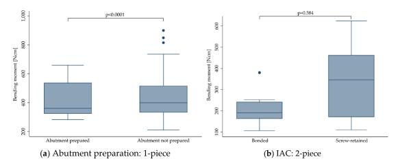
**Figure 7.** Boxplots showing the bending moment at the time point of fracture depending on the abutment preparation for 1-piece (a) and depending on the implant-abutment-connection (IAC) for 2-piece (b) zirconia implants. Whiskers are used to represent all samples lying within 1.5 times the interquartile range. Dots represent outliers. Detailed data can be found in Tables 3 and 4.
