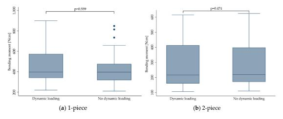
**Figure 9.** Boxplots showing the bending moment at the time point of fracture depending on dynamic loading (Yes: Implants were subjected to dynamic loading, No: Implants were not dynamically
