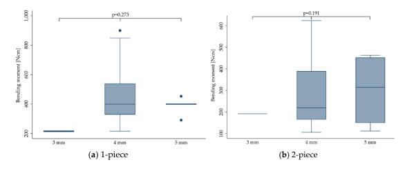
**Figure 5.** Boxplots showing the bending moment at the time point of fracture depending on the implant diameter for 1- (a) and 2-piece (b) zirconia implants. Whiskers are used to represent all samples lying within 1.5 times the interquartile range. Dots represent outliers. Detailed data can be found in Tables 3 and 4.
