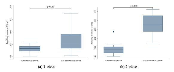
**Figure 6.** Boxplots showing the bending moment at the time point of fracture depending on the crown supply for 1- (a) and 2-piece (b) zirconia implants. Whiskers are used to represent all samples lying within 1.5 times the interquartile range. Dots represent outliers. Detailed data can be found in Tables 3 and 4.
