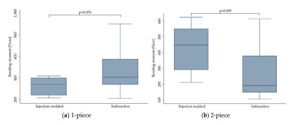
**Figure 4.** Boxplots showing the bending moment at the time point of fracture depending on the manufacturing method for 1- (a) and 2-piece (b) zirconia implants. Whiskers are used to represent all samples lying within 1.5 times the interquartile range. Detailed data can be found in Tables 3 and 4.
