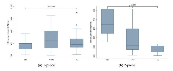
**Figure 8.** Boxplots showing the bending moment at the time point of fracture, depending on the thermal aging conditions (none, HT = high temperature, TC = thermal cycling) for 1- (a) and 2-piece (b) zirconia implants. Whiskers are used to represent all samples lying within 1.5 times the interquartile range. Dots represent outliers. Detailed data can be found in Tables 3 and 4.
