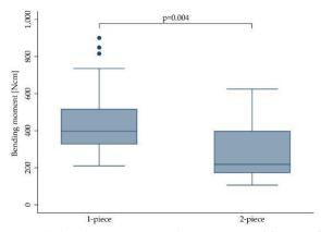
**Figure 2.** Boxplot showing the bending moment at the time point of fracture for 1- and 2-piece zirconia implants. Whiskers are used to represent all samples lying within 1.5 times the interquartile range (IQR). Dots represent outliers. Detailed data can be found in Tables 3 and 4.
