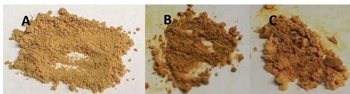
Figure 4.12. Fresh CN-OA-m (A), CN-OA-m after 8 h white light irradiation for standard reaction (B) and CN-OA-m after 48 h green light irradiation for standard reaction (C).
