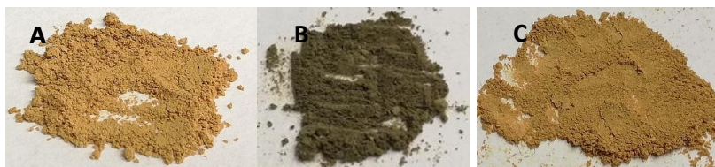
Figure 4.13. Fresh CN-OA-m (A), CN-OA-m after recyclability tests with white light irradiation (B) and CN-OA-m after recyclability tests with green light irradiation (C).
