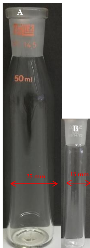
Figure 4.15. Vessel dimensions of vial for scale-up reaction (A) and vial for “standard scale” reactions (B).
