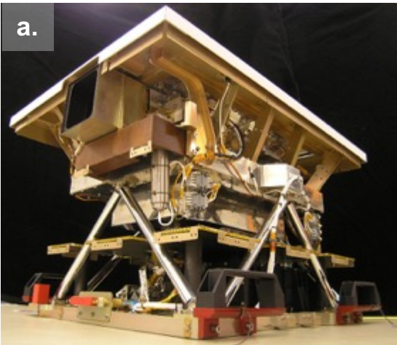
Figure 2.7 Instruments on-board the Dawn spacecraft. (a.) Visual and Infra-Red Spectrometer (Credit: SELEX GALILEO-ASI-INAF), (b.) Gamma Ray and Neutron Detector (Credit: UCLA), (c.) Framing Camera (Credit: MPS). Image source: https://www.dlr.de/content/en/articles/missions-projects/dawn/instruments.html .
