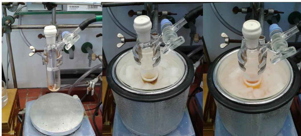
Left: Schlenk tube with ferrocenyl iodide. Center: Solution of ferrocenyl iodide in tetrahydrofuran at -78\text{ }^{\circ}\text{C} . Right: Reaction mixture after adding n -butyllithium.
