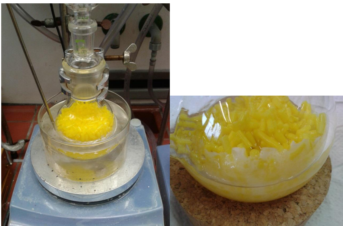
Left: After 1 h, swelling of the filament was observed. Right: Colorless gel deposited on the walls of the flask after cooling to room temperature.
