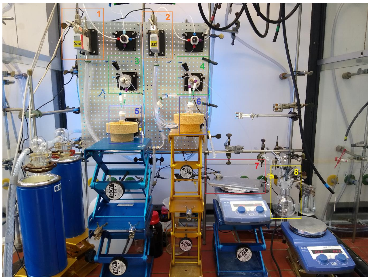
Flow-setup: 1. Mass flow controller 01. 2. Mass flow controller 02. 3. 6-Way valve 01. 4. 6-Way valve 02. 5. Sample Flask 01. 6. Sample Flask 02. 7. Tube reactor with T-piece. 8. Collection flask.
