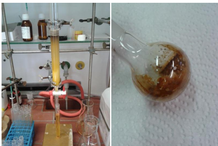
Left: Flash column chromatography of the crude product. Right: Pure product.
