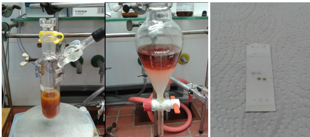
Left: Reaction mixture after stirring at room temperature over night. Center: Aqueous work-up of the reaction mixture. Right: TLC of the reaction mixture after aqueous workup (left lane: starting material, middle lane: co-spot; right lane: crude product; vis. vanillin).
