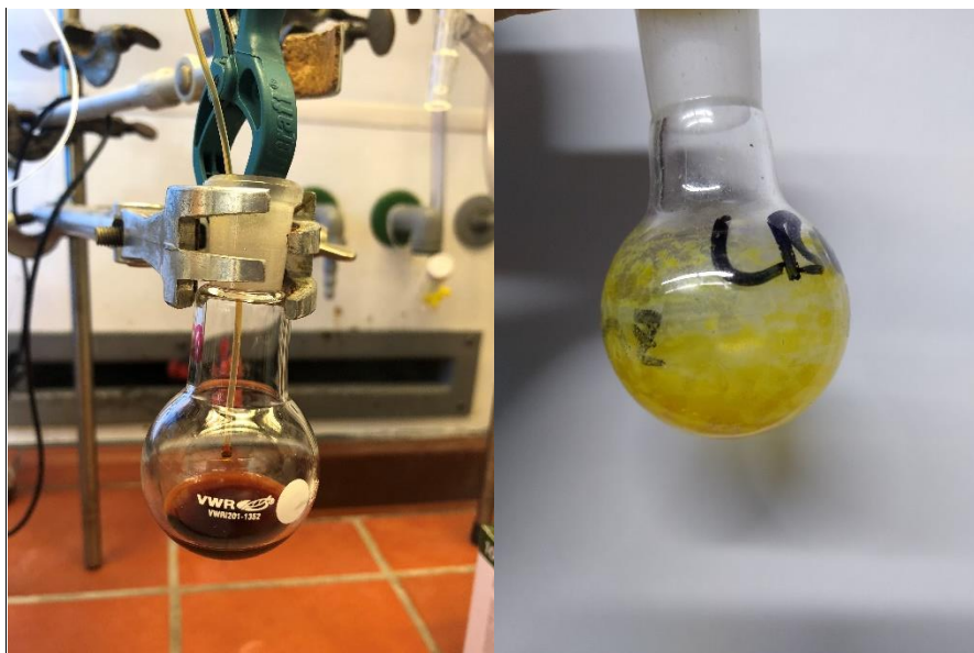
Left: The crude product solution after passing through the heated tube reactor. Right: The isolated product 3b .
