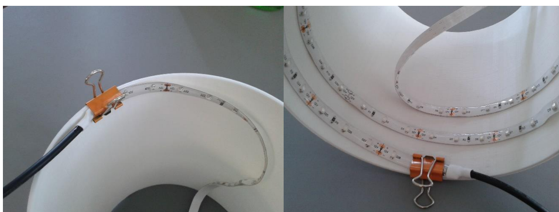
Left: The LED stripe is secured with a clip on the top of the body of the photoreactor. Right: The LED stripe is coiled inside of the body.
