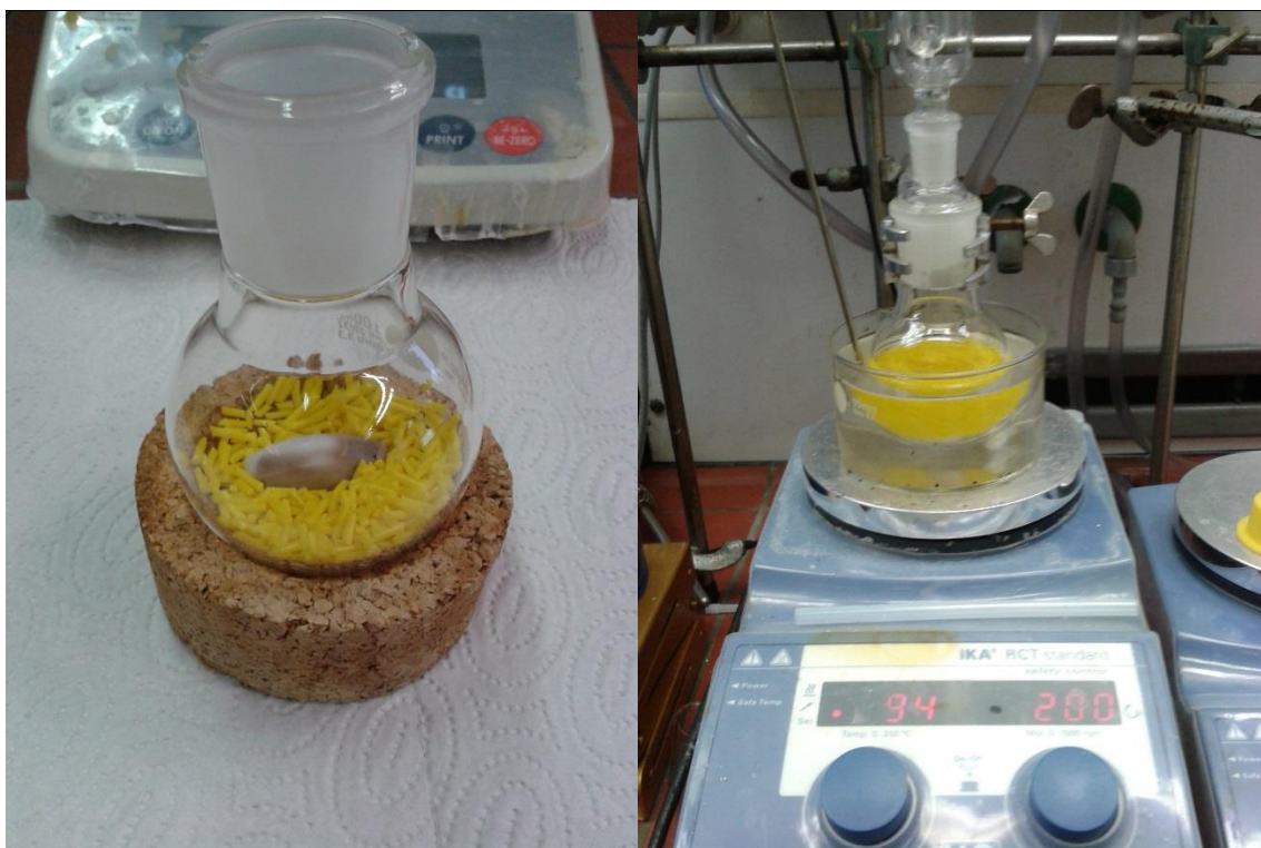
Left: The cut filament before treatment with THF. Right: Boiling the filament in THF.
