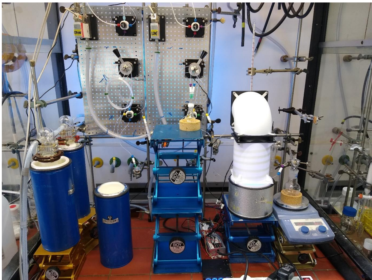
The flow setup for the photochemical gram scale C–H chlorination of (+)-sclareolide (9).
