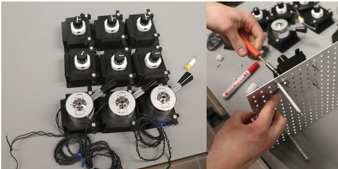
Left: A small collection of the three different valves placed in the valve sockets. Right: The sockets are mounted on the controller board using M4 screws.
