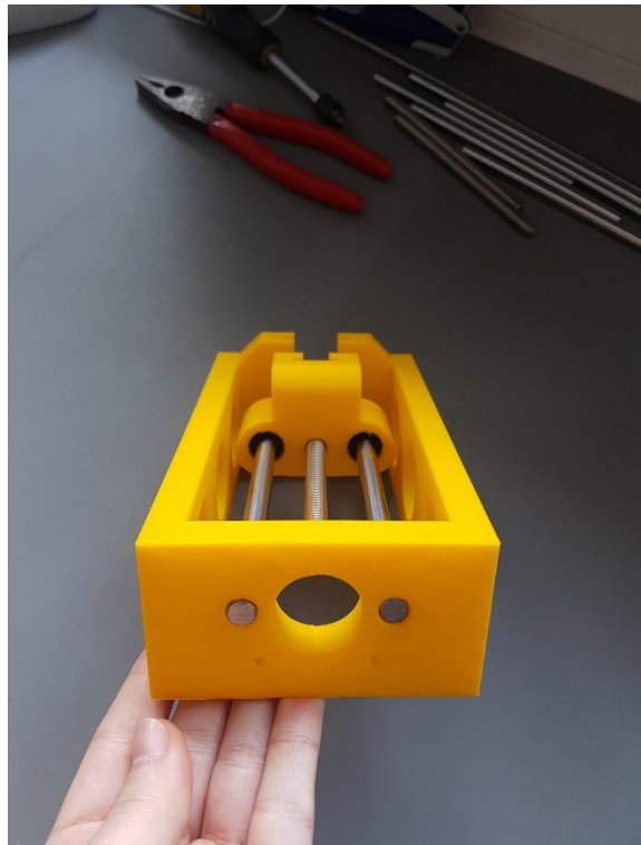
Left: The sledge with the linear rods and a M8 threaded bolt in the middle. Both the threaded bolt and the linear rods were shortened by a jab saw. Right: The sledge placed in the body of the syringe pump.
