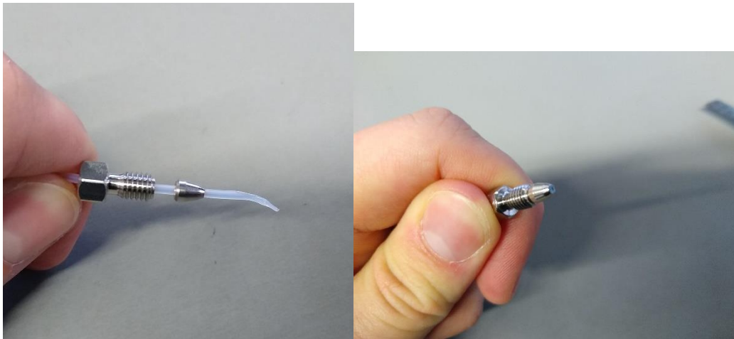
Left: In the same way, tubes (outer diameter 1/16") are equipped with HPLC fittings (10-32 UNF fitting) and conical ferrules Right: A tube equipped with fitting and ferrule.
