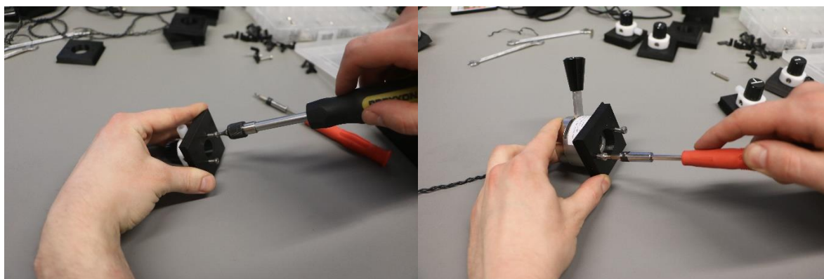
Left: The low-pressure valves are secured on the low-pressure valve mounts using M3 screws. Right: The HPLC injection valves are secured on the corresponding mounts using M4 screws.
