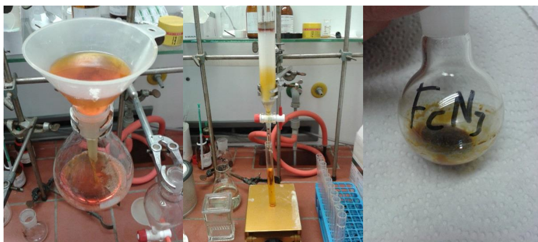
Left: Removal of the drying agent by filtration. Center: Gravity column chromatography of the crude product. Right: Pure product.
