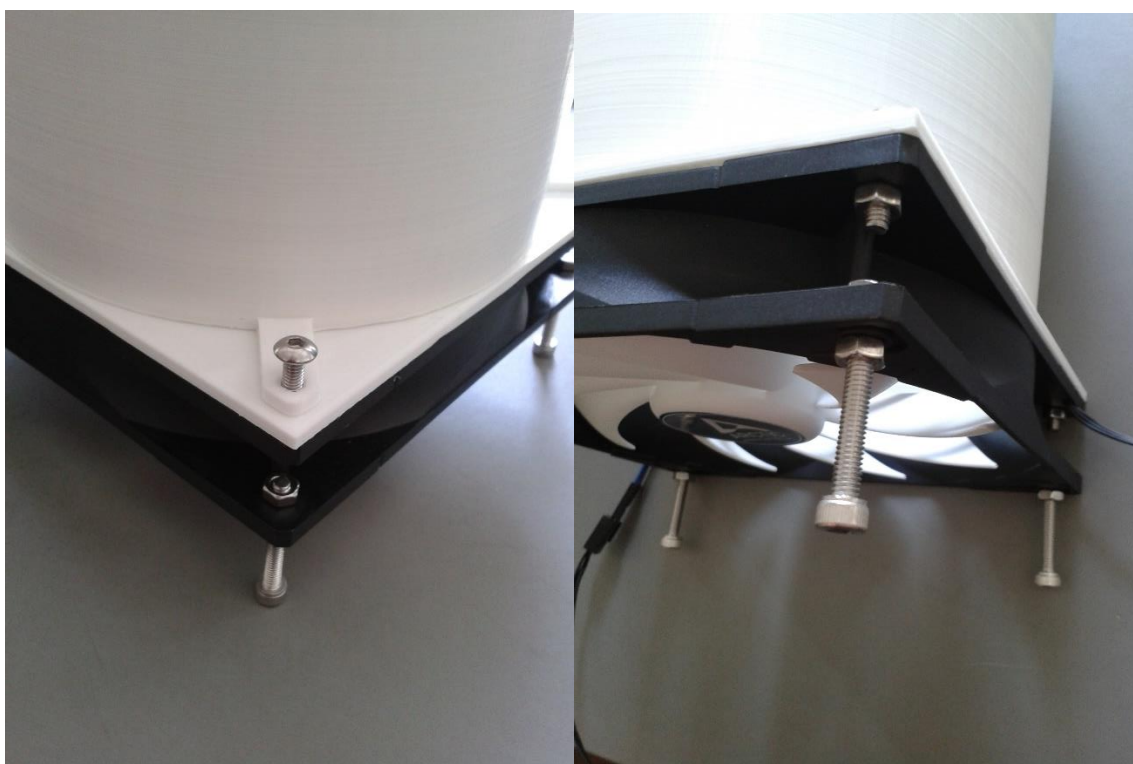
Left: The bottom plate and the fan are connected with a M4x16 screw. Right: The fan is equipped with a M4x30 screw. These screws serve as “foots” for the photoreactor to allow a proper air stream for the fan.
