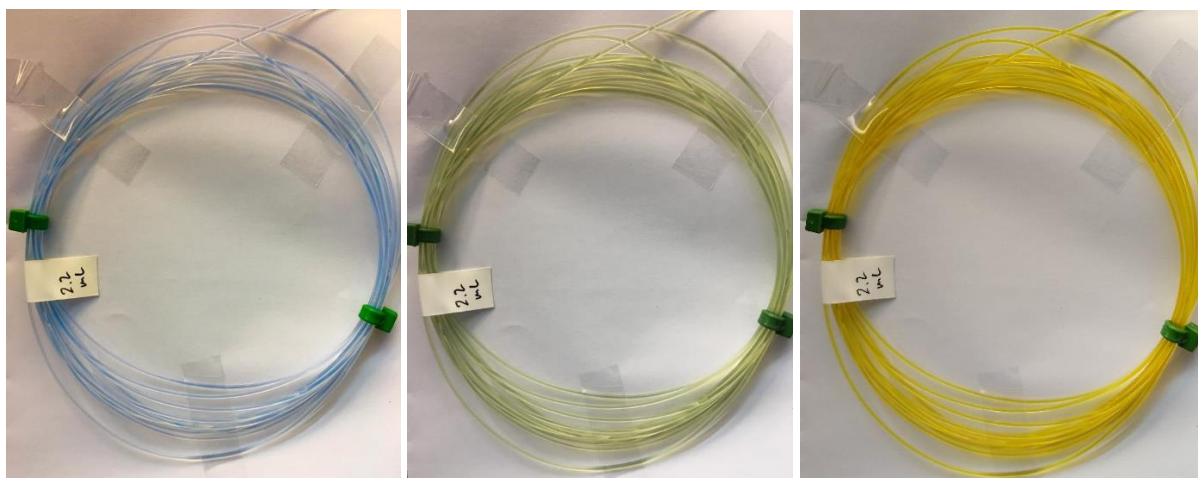
Left: The indicators solution ~30 seconds after loading on the sample loop. Center: After 30 min. Right: After 60 min.
