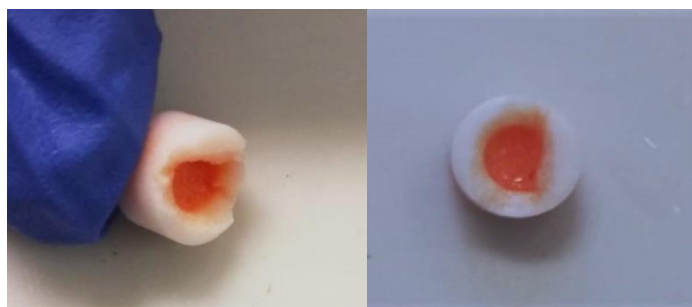
Figure 28. Pulsatile release tablets first formulation after 18 hours of dissolution test in HCl 0.1 N, pH 1.2.
