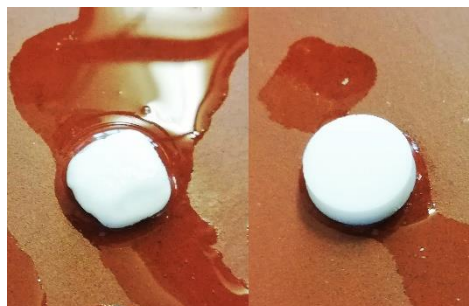
Figure 17. Matrix tablets containing Ethocel 10FP, 20% (left) and 35% (right), respectively, after 24 hours of dissolution test, at 50 rpm.
