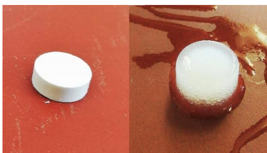
Figure 13. Matrix tablets containing Methocel K15MCR before (left) and after (right) dissolution test at 50 rpm.
