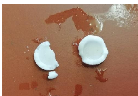
Figure 30. Pulsatile release tablets with coating layer of Compritol ATO 888 after rupture, during dissolution test.
