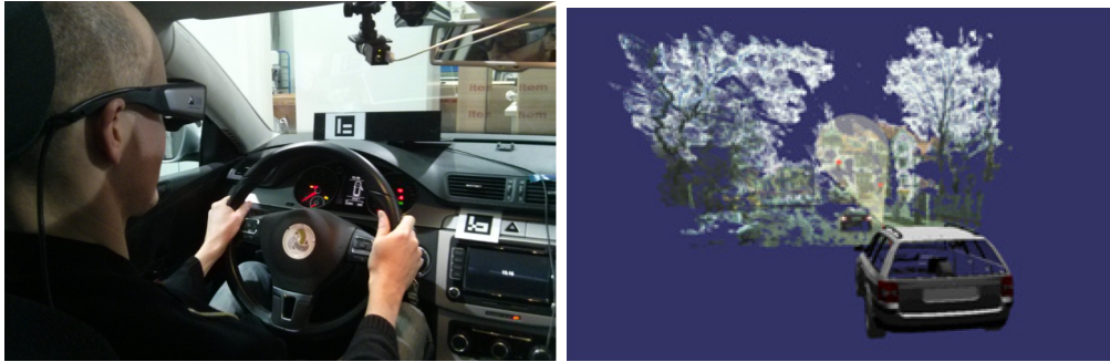
Figure 13: Left: The driver is wearing eye-tracking glasses from SMI, a camera in the glasses is perceiving the fiducial markers and localizes the head relative to the car. Right: The depth and image information of the stereo camera is projected as a colored point cloud into the 3D space with respect to the car.
