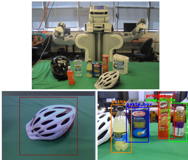
Figure 9: Top: Demo setup with PR2 and objects to detect in front of it; Bottom left: Training user interface, object to learn in region of interest (red square); Bottom right: Detected objects in bounding boxes.
