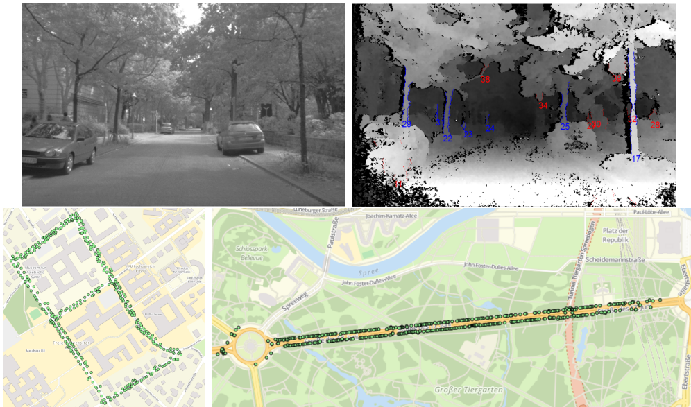
Figure 14: Upper left: Rectified image from the FU campus; Upper right: Depth image with recognized trees; Lower left: Tree map from FU campus, Takustraße; Lower right: Tree map of Straße des 17. Juni.
