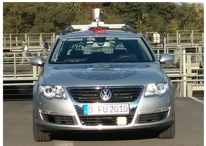
Fig. 1. Test Car MadeInGermany from Freie Universität Berlin, the Kinect devices were placed on top of the roof, in front of the Velodyne HDL 64 lidar sensor.
