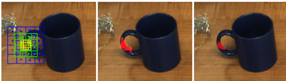
Figure 10: Local grasp region detection for a cup object. Left and center: SIFT descriptors on a key point were used to find suitable gripping points for the PR2 robot. Right: The point region is smoothed.
