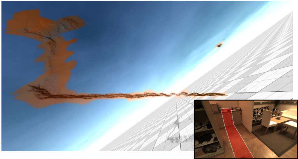
Figure 4.1: Visualization of Point clouds using AIT Stereo Vision from an indoor environment from the marked area. The cloud is shown from the side, the tilt from the camera (red) was removed. The transparent ellipsoids represent the uncertainty of the non-transparent point clouds
