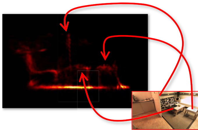
Figure 4.27: Overview of the data in a histogram from AIT Stereo Vision and real image. The orientation has been removed since the Manhattan system geometry is known
