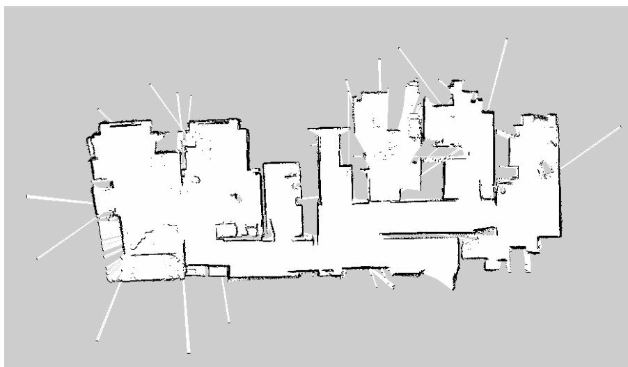
Figure 2.12: SLAM map of the environment using the gmapping package and two SICK laser scanner
