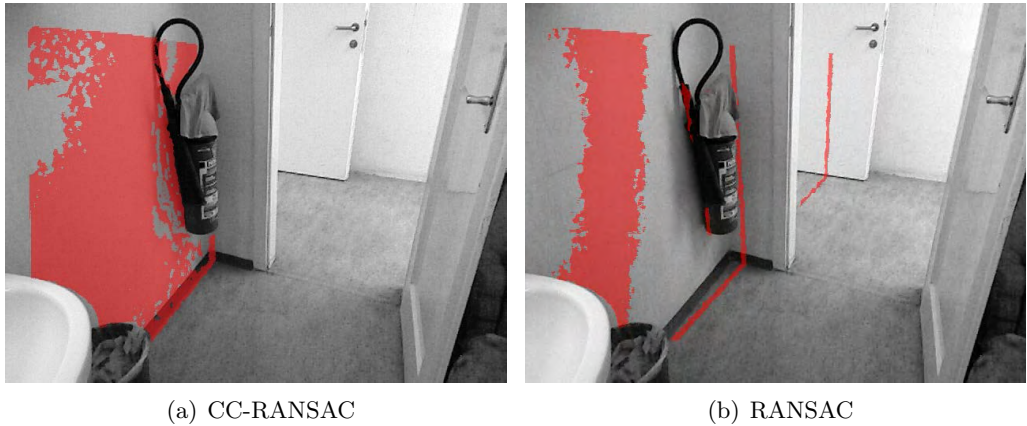
Figure 4.23: Comparison of Plane estimation using CC-RANSAC and standard RANSAC using normal vectors, no least square fit, 16 estimation iterations and 5cm distance threshold to the plane model
