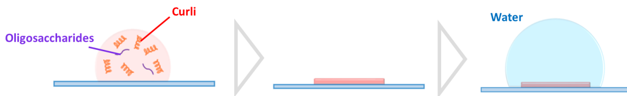
Figure 4-13. Cartoon representation of the sample preparation method.
