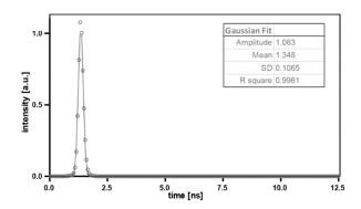
*Fig.* 13: Normalized instrument response function of TCSPC. Measured by SHG of KDP crystals. Red circles: data points, blue line: Gaussian fit (Suppl. Fig. S6 B in [Leben et al., 2018]).
