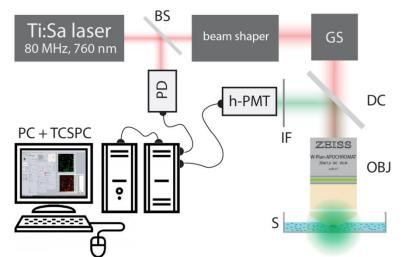
*Fig. 12:* Schematic two-photon microscope setup to perform time-domain FLIM. BS (beam splitter), GS (galvo scanner), DC (dichroic mirror), OBJ (objective), S (sample), IF interference filter), h-PMT (hybrid-PMT), PD (photon diode), PC (personal computer), TCSPC (time-correlated single photon counter. (Scheme taken from (Leben et al. 2018)).
