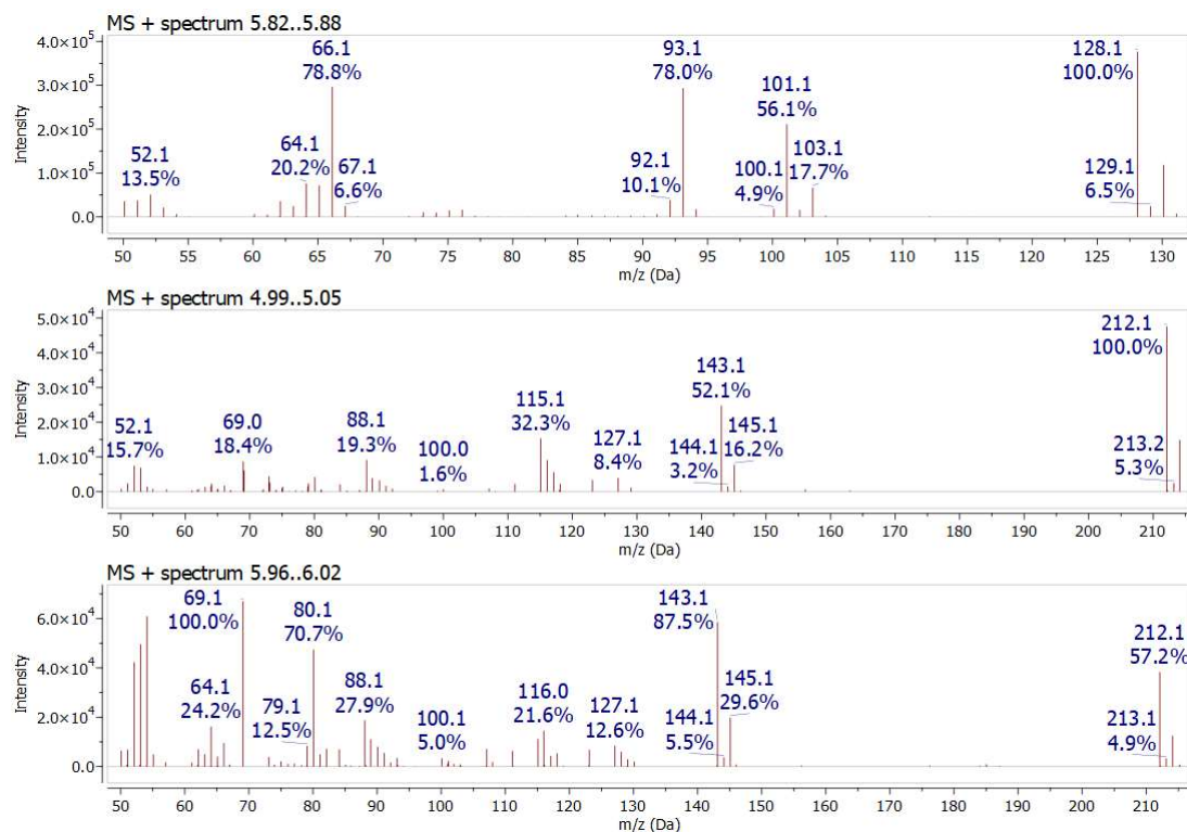
Figure S115. GC-MS spectra of a reaction mixture, prepared by method B (3 mmol scale, 0.2 M) using 6-chloropyridin-2-amine ( 4f ) as substrate, showing 6-chloropyridin-2-amine ( t_r = 2.04 - 2.12 ) and two distinct 6-Chloro(trifluoromethoxy)pyridin-2-amines ( t_r = 4.99 - 5.05, 5.96 - 6.02 ).
