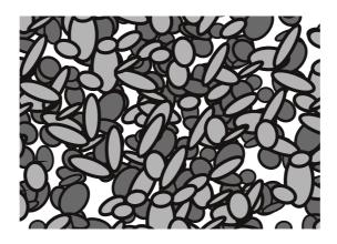
Figure 1.1: Simplified illustration of rocks on the grain scale. The pore space (white) in between the rocks solid constituents (grey) is in-situ filled with fluids (liquid or gaseous).
