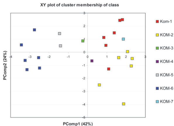
Fig. 14 Principal component analysis of the results of WD-XRF analysis (Si, Ti, Al, Fe, Mg, Ca, Na, K, Sr, and Zr) of glass samples from Komariv.
