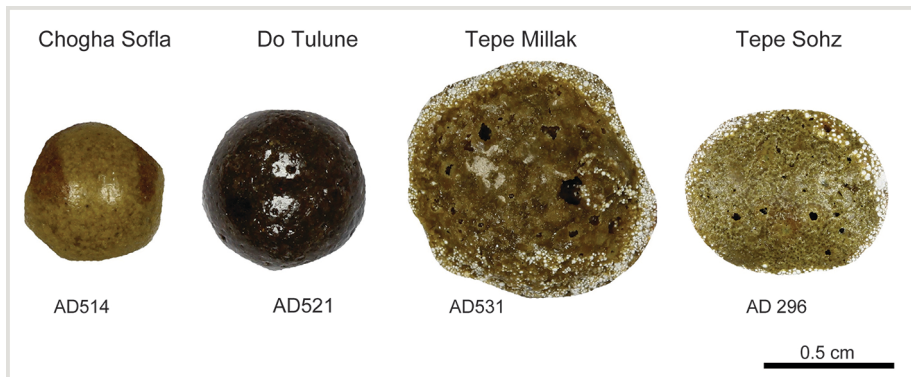
Fig. 6 Distinction of pottery from different sites by refiring at 1200°C (project: Tepe Sohz).
