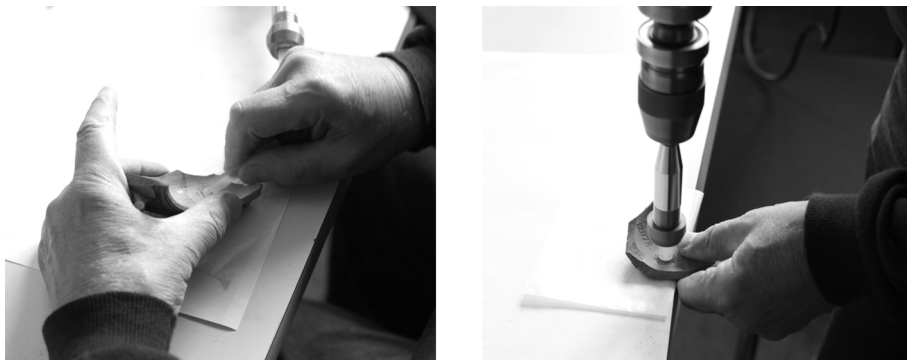
Fig. 1 Cleaning and extraction of sample by drilling.
