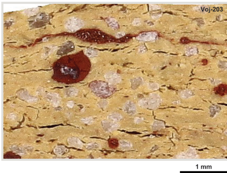
Fig. 16 Alteration effect through infiltration of iron-rich solutions into sherds clearly visible after refring at 1150°C.
