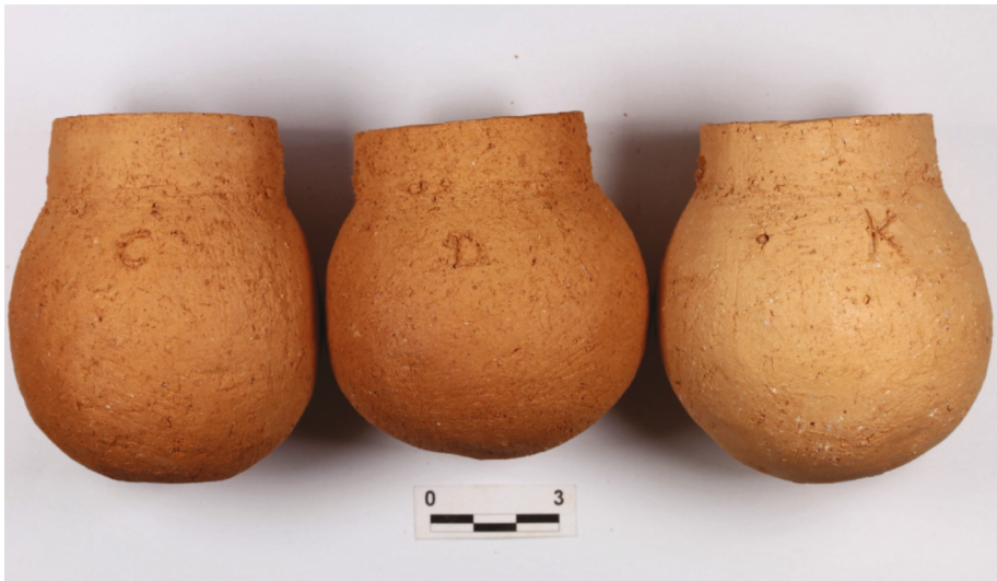
Fig. 10 Vessels produced and used for the model analysis to assess functional properties (water permeability). Different tempers were added: C = cow dung, D = donkey dung, and K = kaolinitic sandstone.
