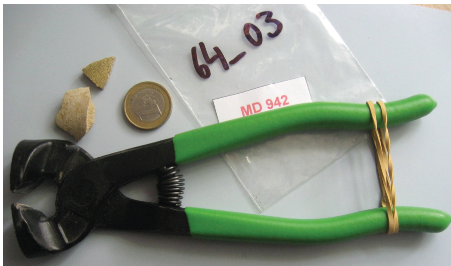
Fig. 7 Pliers with tungsten carbide cutting edges (used for mosaics) for optimal use in knapping pottery samples or producing fresh fracture surfaces for macroscopic description or pXRF measurements.
