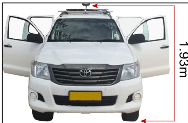
Fig. 6 Measurement setup—Toyota Hilux with GS 16 sensor on the car roof (photo and editing: Robert Arendt 2018)
