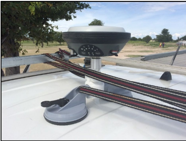
Fig. 5 Leica GS 16 Sensor installed on the roof of a car (photo: Robert Arendt 2018)
