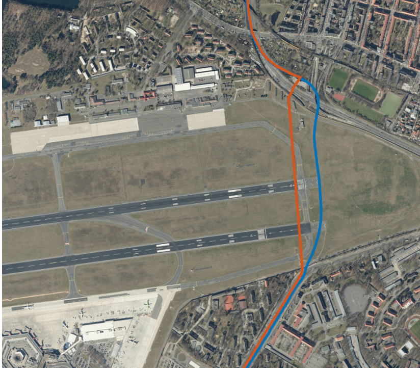
Figure 7.2.: A detailed view to the path during the GNSS blackout inside the airport tunnel. The estimated path follows the actual path on lane, while GNSS signal shows a jump between tunnel entrance and exit.
