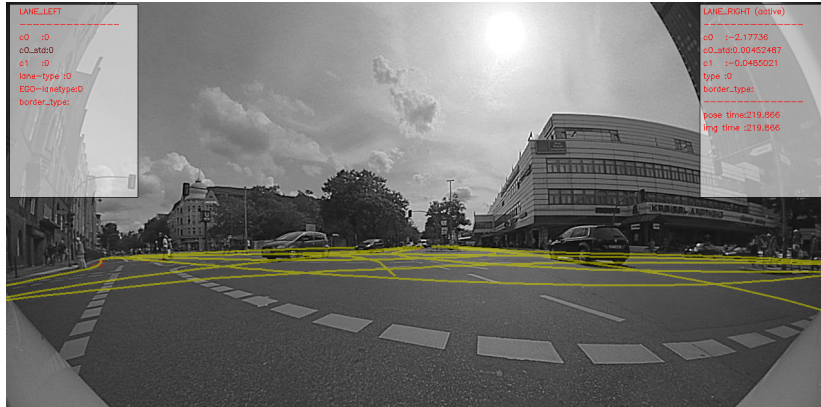
Figure 6.23.: A crossing scene in practice. Reprojected map lane segments shown in yellow. Information from lane measurement is shown inside the highlighted boxes.
