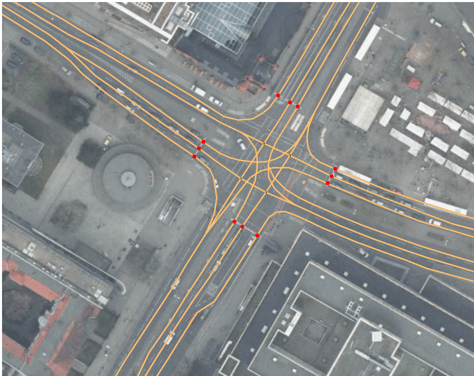
Figure 5.3.: Illustration of the extended OSM-data at a multi-lane-crossing. All lanes are modeled separately with the use of the lane-middle-path. The stop lines intersections with lanes are shown as red diamonds. Connections on (multiple)turning lanes are modeled in a way, that they describe a natural path and according to guidance-markings, if available.
