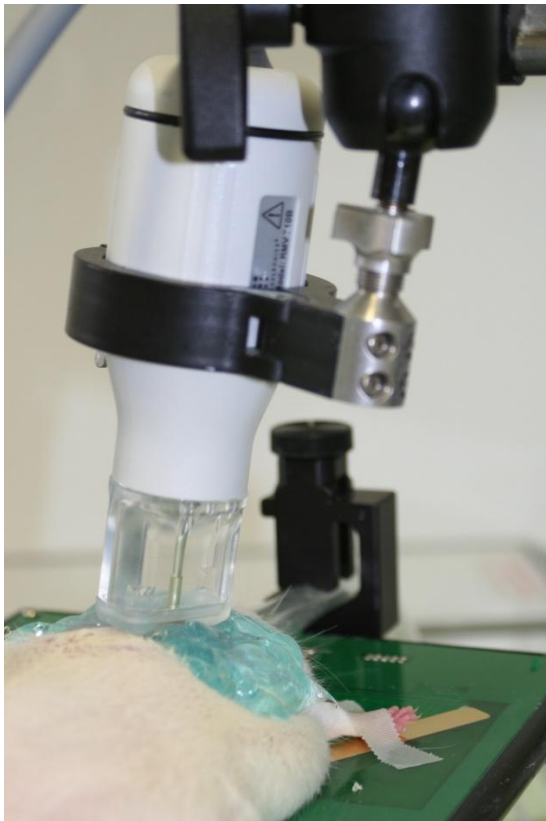
Figure 9: A high-resolution imaging echocardiography system Vevo 770 (VisualSonics Inc., Toronto) equipped with a 25 MHz single-crystal transducer.
