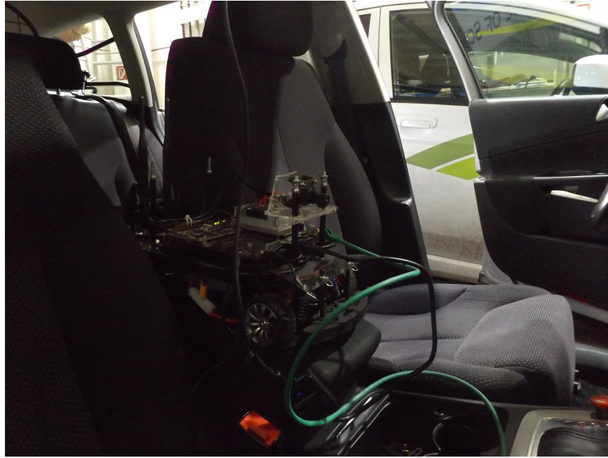
Figure 48: AutoMiny Tx1 mounted in the MIG to record the dataset, the car is connected through Ethernet to the MIG.
