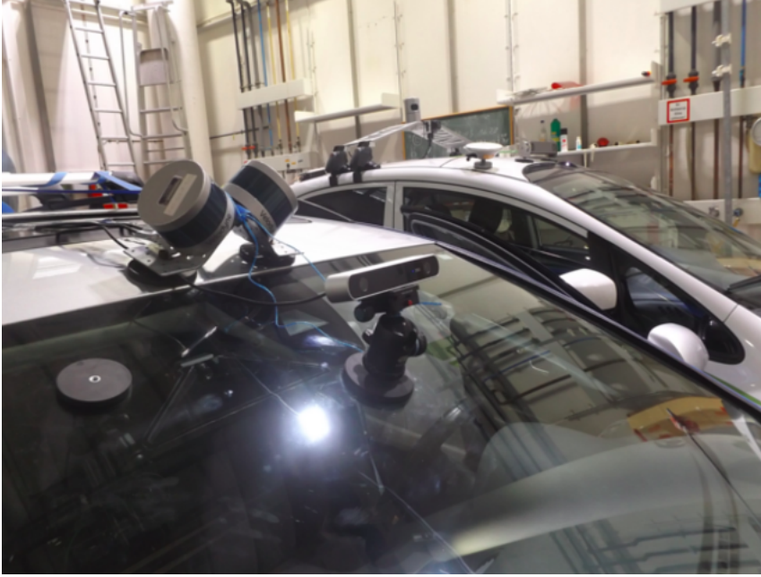
Figure 47: ZED camera mounted on the MIG windshield.
