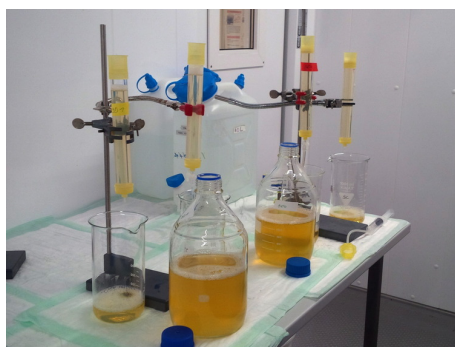
Figure 9: Harvest of secreted protein from insect cell media using IMAC at 4 °C.
