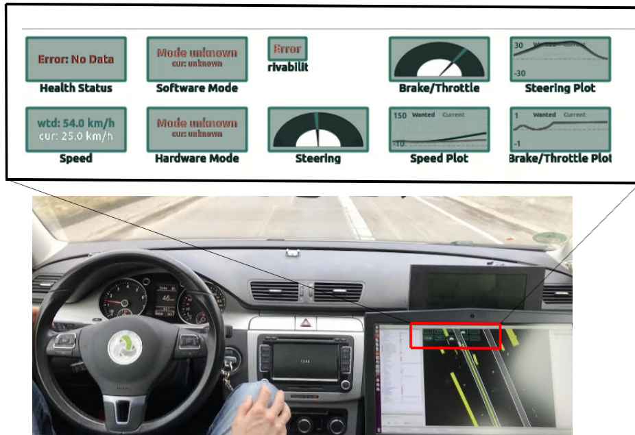
Fig. 2.7: Status Monitoring: health status, software and hardware mode, autonomous drivability, real and planned speed, steering and accelerator/brake pedal position.
