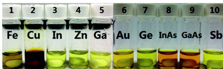
Figure 25. Mixtures of the ILs and the metal chlorides after complete dissolution of the corresponding metals or alloys. [149] Reproduced from Ref. [149] with permission from the Royal Society of Chemistry.
