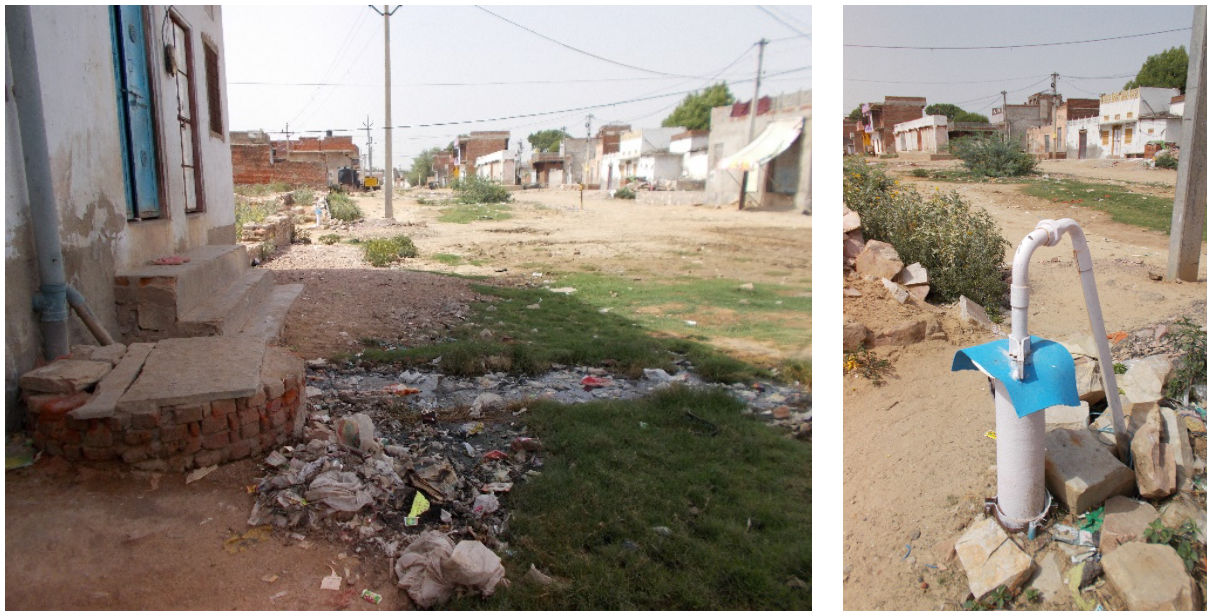
Fig. 11: Typical, unpaved street of Nai Ki Thari, July 2015, with septic tank (left), grey water outflow, solid waste disposal and drinking water production well (background and right side).
