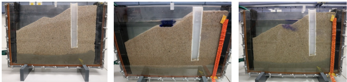
Fig. 57: Physical Groundwater Model developed in frame of the project. The picture on the left shows the model in normal condition. In the middle, a surface water contamination is represented by adding ink to the surface water body. Due to pumping in the deep well, a contamination plume can be seen on the right picture. Photos taken by Christoph Brüdigam.
