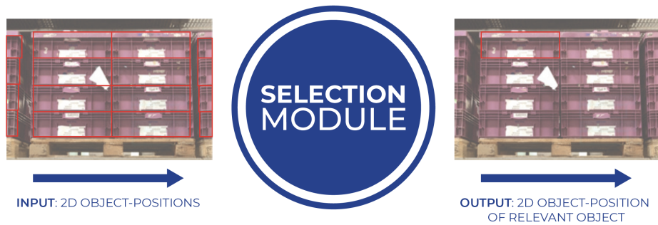
Figure 4.28: Target-specification for the Selection-Module (own illustration)
