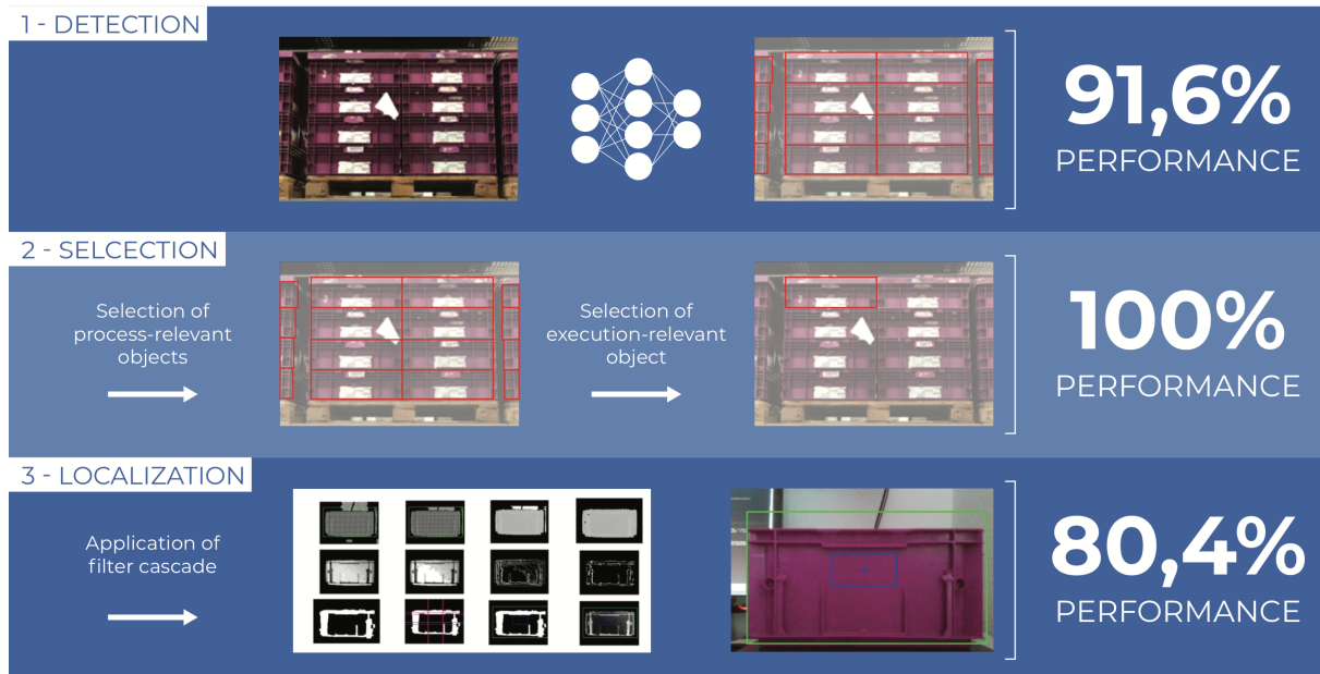
Figure 4.55: Summary of the evaluation of the Perception Algorithms functional modules (own illustration)
