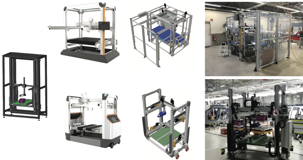
Figure 3.8: Robot for handling full containers: draft, construction, prototype, serial version (own illustration)
