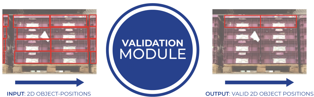
Figure 5.10: Target-specification for the Validation-Module (own illustration)
