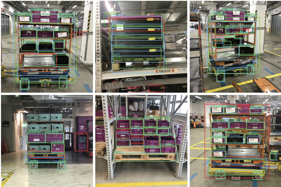
Figure 5.2: error clusters: blue - ground truth, green - correct detections, errors - red (own illustration)
