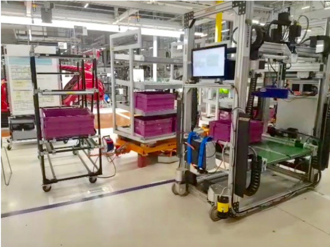
Figure 6.3: Provisioning robot in real plant logistics area (Leipzig) (own illustration)
