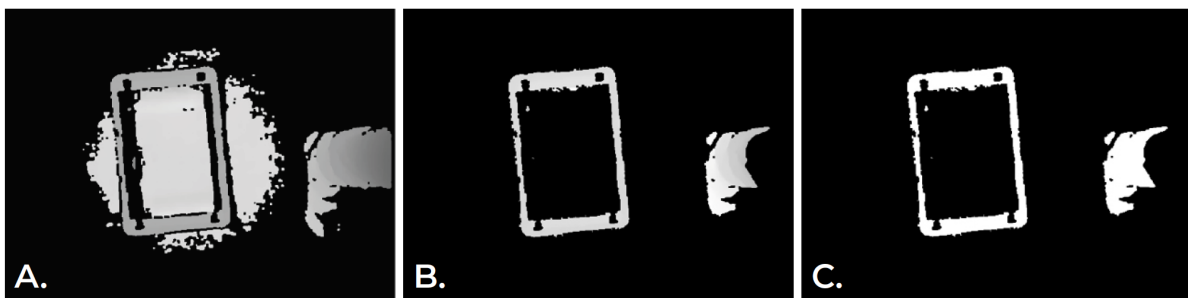
Figure 4.39: Foreground background separation by thresholding (own illustration). A) Smoothed Image, B) Image after the application of lower and upper thresholds, C) Final image after setting all pixel values in those bounding boxes to 1.
