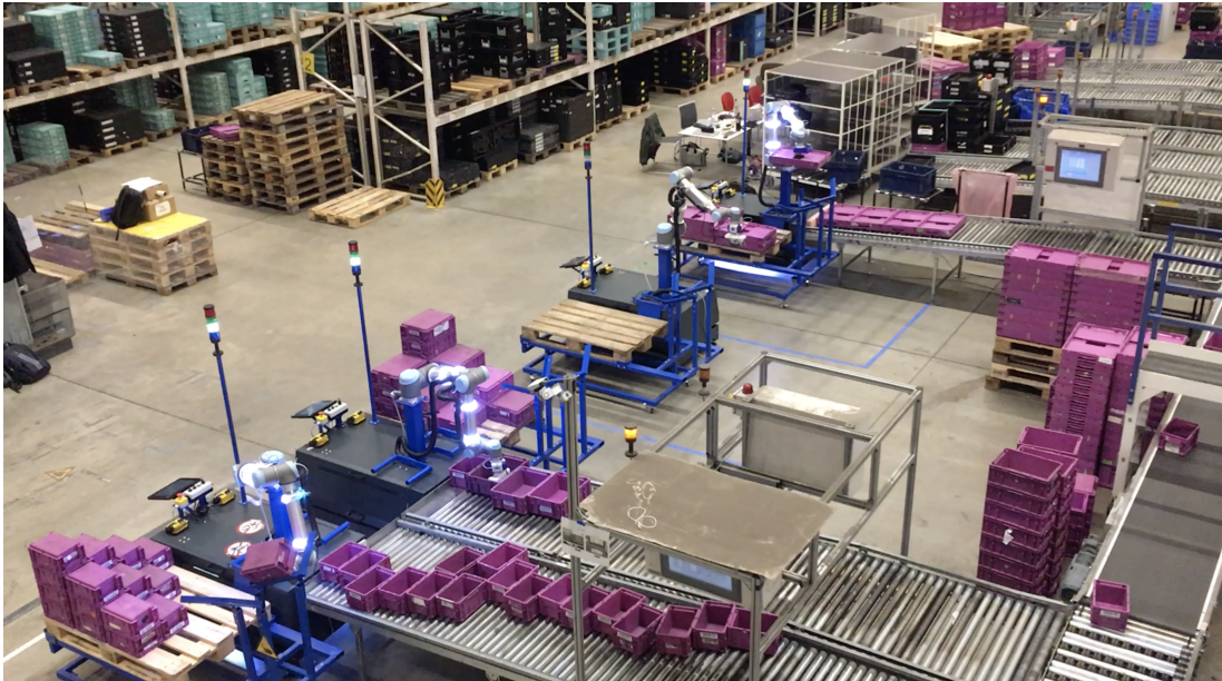
Figure 6.1: Palettizing robots working productively in serial processes of the plant Leipzig (own illustration)
