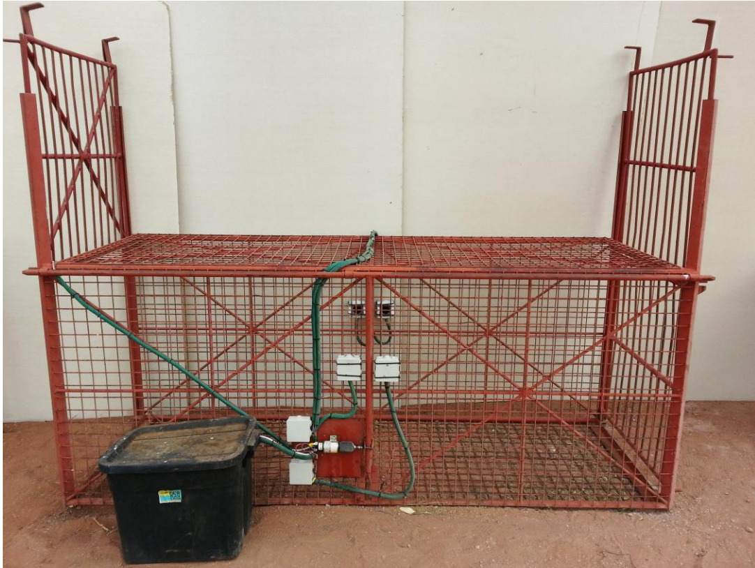
Figure 1: Boxtrap with sensors mounted in the white boxes on the sides of the trap. Black box contains 12V battery and the circuit board (see Figure 2) in a water proof housing.
