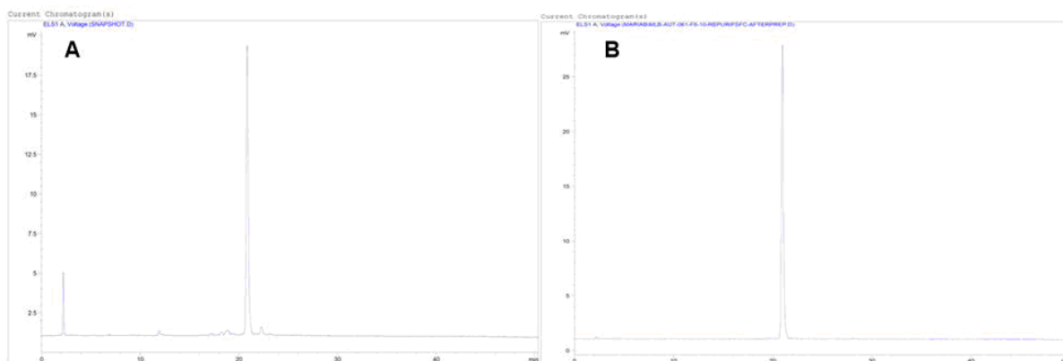
Analytical NP-HPLC of (A) crude reaction mixture after photocleavage and (B) the purified product. Detection: ELSD.
