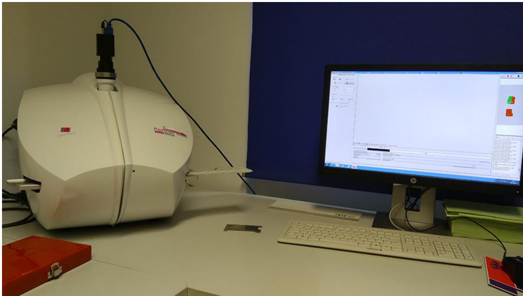
Figure 2.2: Pannoramic™ Digital Slide Scanner (Pannoramic™ MIDI II). The scanner scans automatically up to 12 slides in one run and supports the Carl Zeiss objectives.
