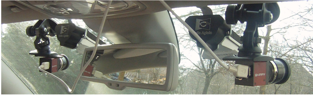
Figure 5.1: Two AV Guppy F-036C cameras were mounted with suction cups behind the windshield. The camera are pointed slightly upwards and sideways to maximize the covered field of view for close-range traffic light detection.
