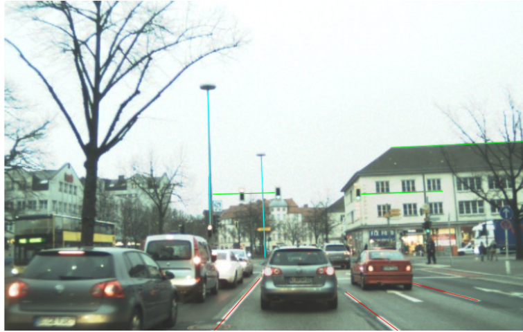
Figure 3.4: Single-image calibration from parallel lines. The lane markings yield the car's x-axis (red), the building's roof and windows the y-axis (green), and the lamp posts the z-axis (cyan).
