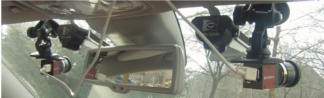
Figure 1.2: Two AV Guppy F-036C cameras were mounted with suction cups behind the windshield. The camera are pointed upwards and sideways to maximize the covered field of view for close-range traffic light detection.
