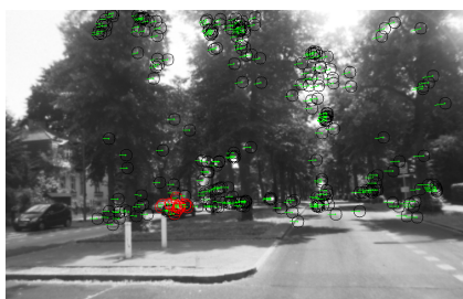
(a) The approaching vehicle perturbs the ego-motion flow.
