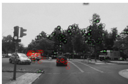
(b) Optical flow separates stopped cars from moving cars.
