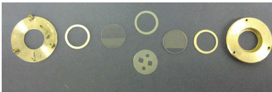
Supplementary Figure 8: Home built cuvette for acceleration and photolithography measurements. Two different spacers were tested: (i) One spacer exhibits two chambers filled with the same sample. One of the chambers is excited with IR light, the other one is not illuminated. (ii) One spacer exhibits only one big chamber. Here, two identical samples and cells were used, one was excited with IR light, the other one was not.
