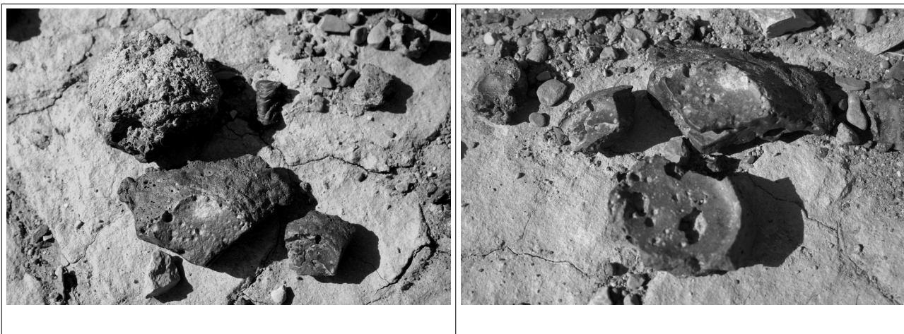
Figure 53: Several bottom fragments of crucible slags from the 3rd millennium BCE metallurgical site at Shahdad (with the courtesy of M. Vidale).
