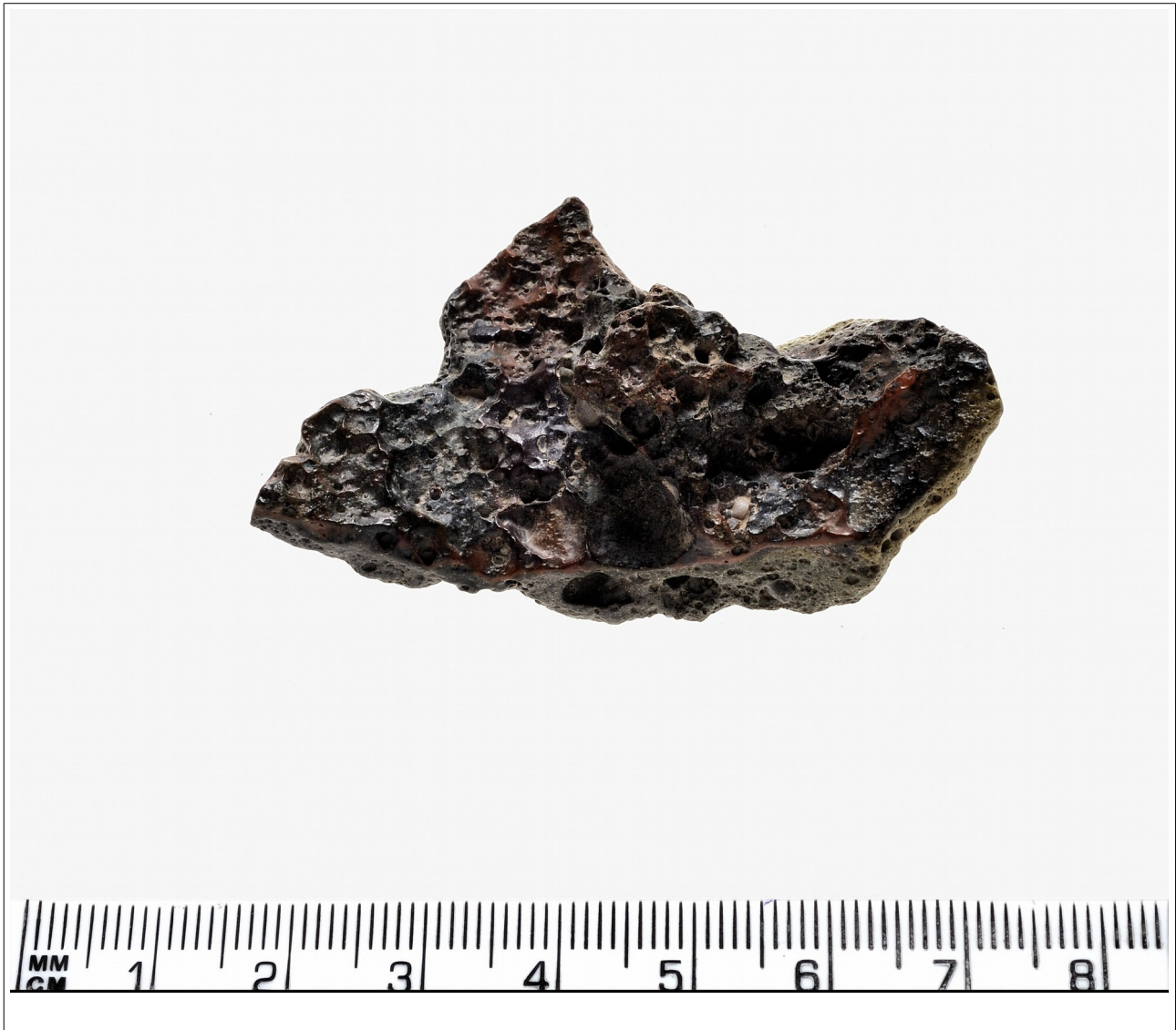
Figure 58: Fragment of a furnace lining SHA 2 (Photo by E. Loliva).
