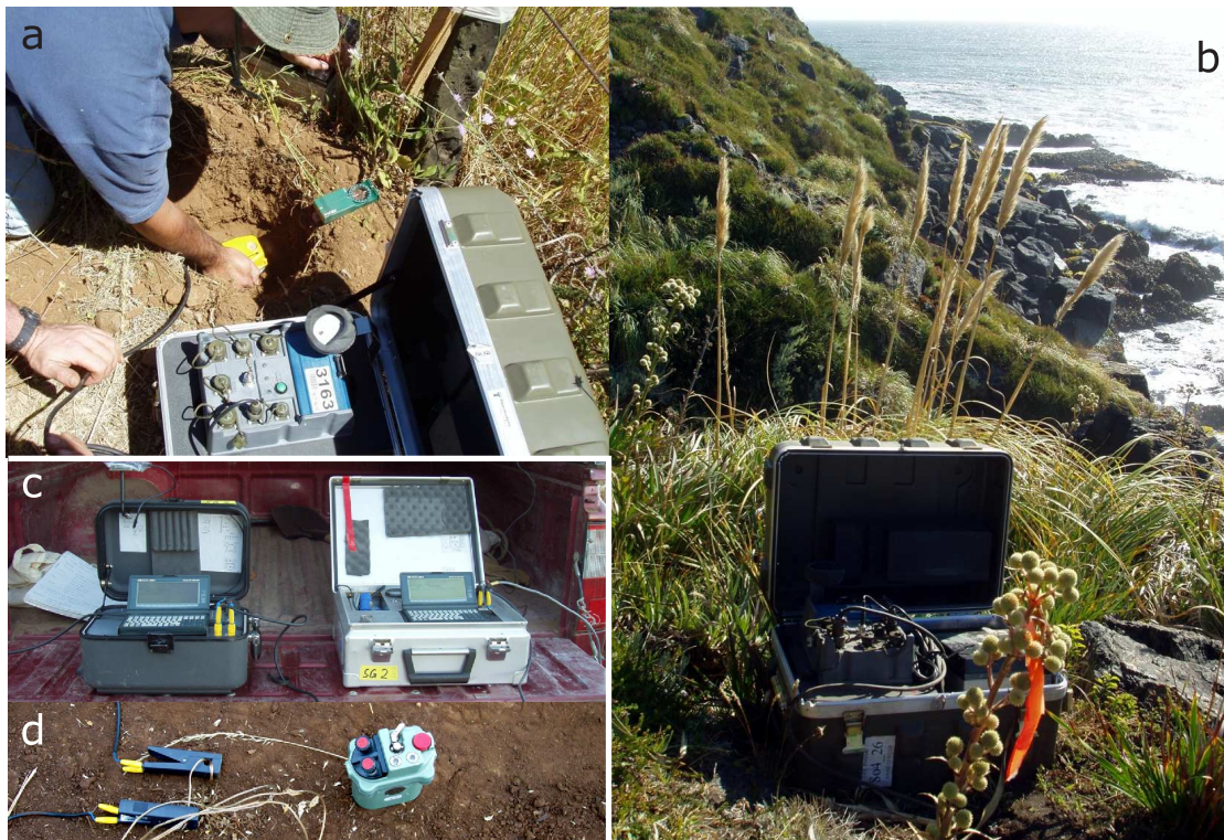
Figure 2.4.: Receiver stations and shooting equipment. Panel a shows the buried and oriented 3-component geophone and the EDL recording unit in a weatherproof box. The picturesque last receiver station 955 at the Pacific Ocean is shown in b. Panel c shows two similar boxes to record the exact shot times, e.g., with pliers around the ignition lead, not yet connected to the trigger box (d). Image courtesy of C. Krawczyk.
