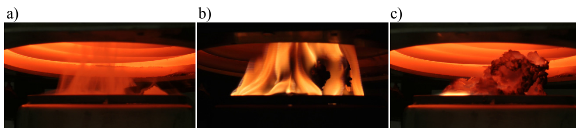
Figure 4.2.9 Fire behaviour of PC/ABS PTFE + HDP under forced flaming combustion in the cone calorimeter: a) before ignition, with the release of pyrolysis products and the shrinkage of the polymer b) during combustion with flame covering the whole sample and formation of a char “tower” c) char residue after extinction
