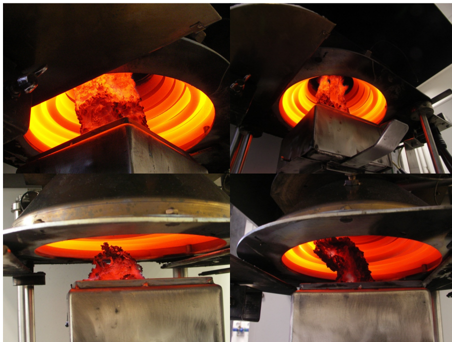
Figure 5.1.10 Action of DPZ flame retardant by enhancement of the char formation by an intumescence process: PC/8DPZ (top left) and PC/8DPZ PTFE (top right), PC/ABS PTFE without flame retardant (bottom left); PC/ABS/8DPZ PTFE (bottom right); in the cone calorimeter (50 or 70 kW m -2 ) after flame out
