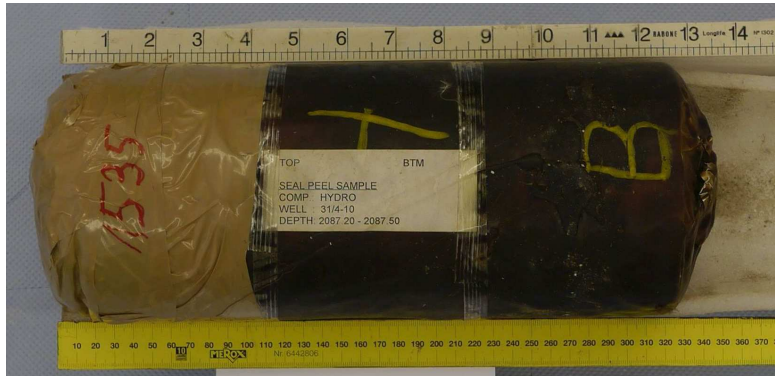
Figure 6.8: Seal peel sample SPS, income state. The core was preserved by three layers: resin, steel, gyps. Photo is provided by the "Gesteinslabor Jahns" laboratory.
