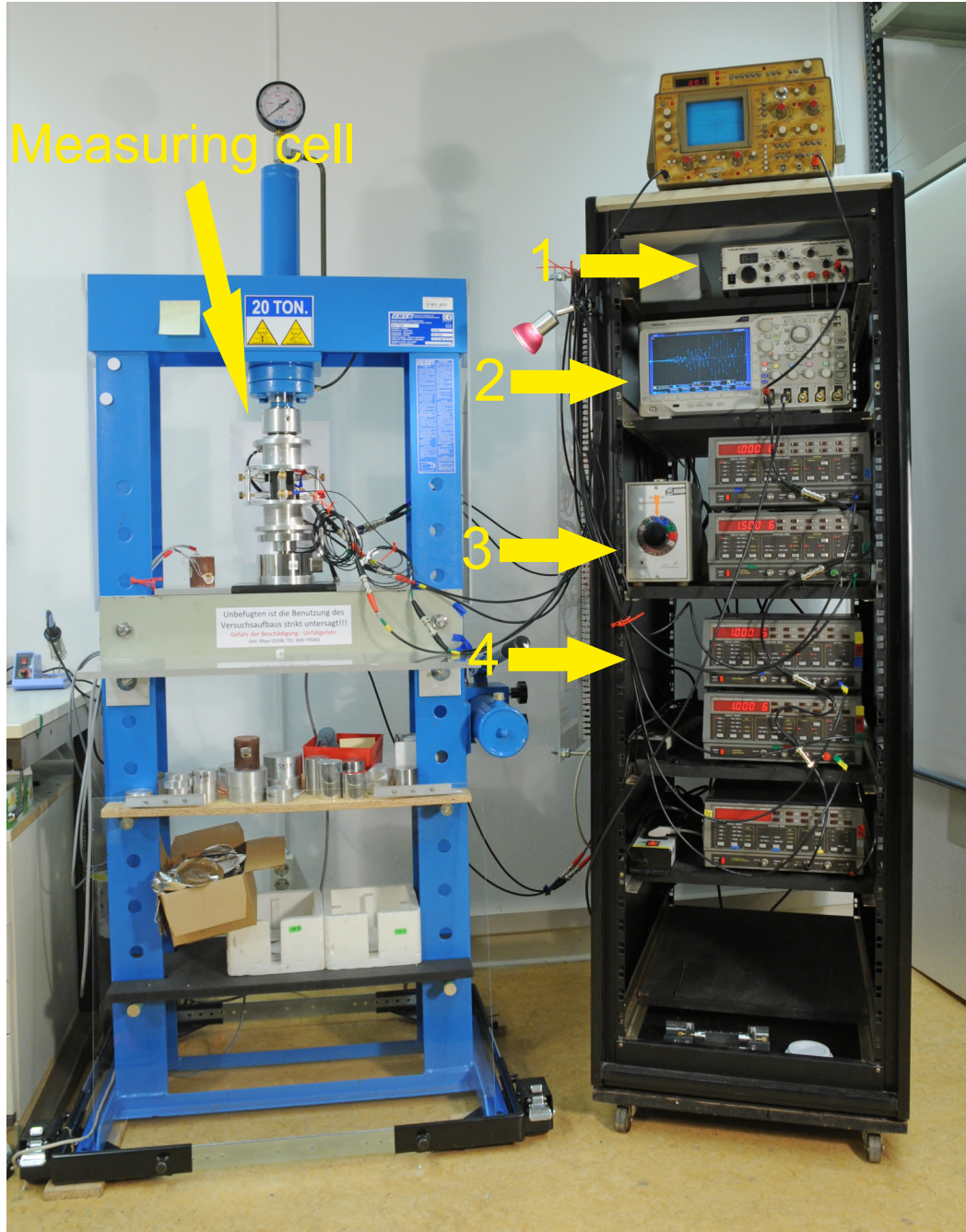
Figure 3.6: Left: the hydraulic press with mounted measuring cell and the sample. Right: 1 – the trigger, 2 – the oscilloscope, 3 – the control device, and 4 – the generators. Photo provided by Jan Evers.
