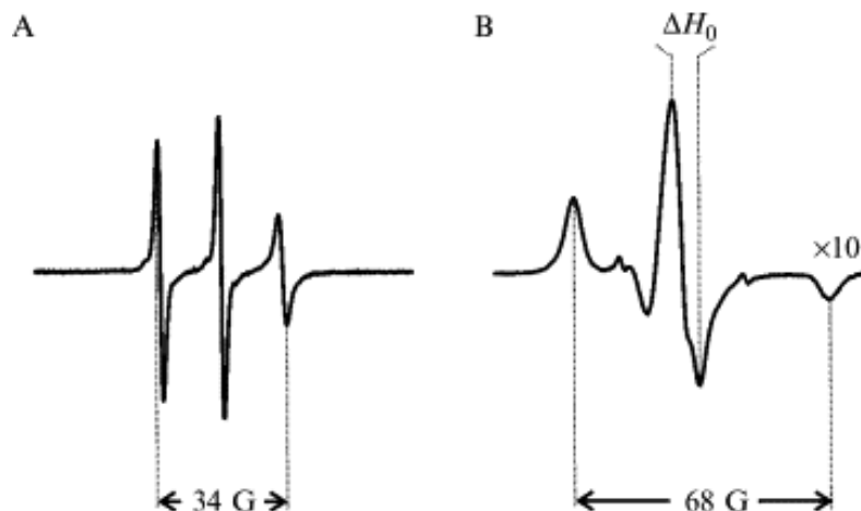
Figure 47: Mobility of R1 determines electron paramagnetic resonance spectral line shape. A test protein is spin-derivatized at a single position. A Three sharp peaks indicate high mobility in the GdnHCl denatured state. B Broad, highly separated peaks and small amplitudes reflect low mobility of the buried spin label in the native fold ([236]. For a comparison of line shapes, the spectrum in B is amplified 10-fold. The scan width for both spectra is 100 G. Dotted lines mark outer peaks. Separation between outer peaks is indicated for both spectra. The peak-to-peak distance of the central resonance, defined as the central line width ( \Delta H_0^{-1} ), is indicated in B. Figure and legend adapted from [195].
