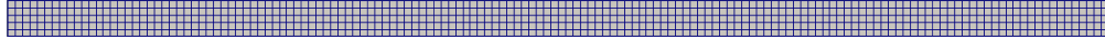
Figure 6.2: The computational mesh consists of 750 considerably stretched rectangular grid cells, aligned in five layers. The graphic above is scaled by a factor 500 in radial direction.
